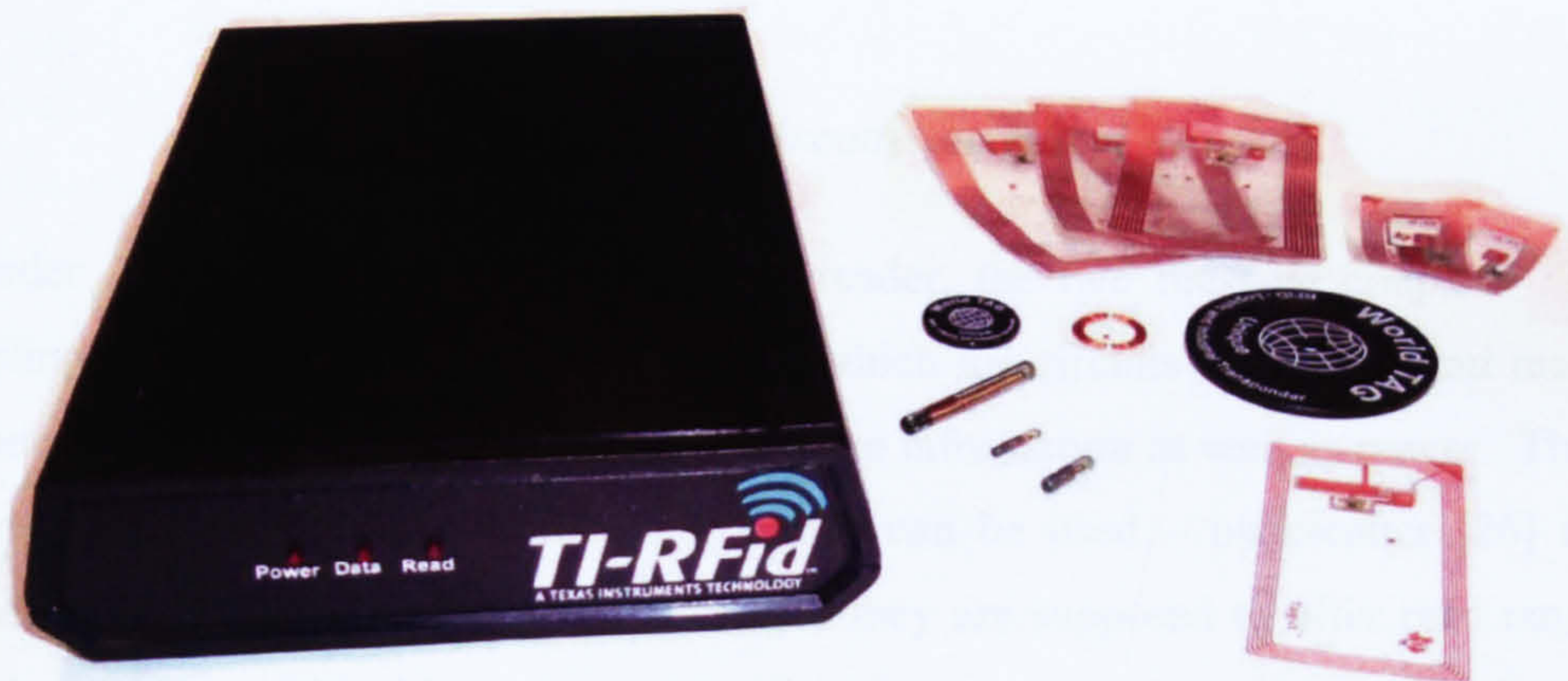
Figure 2.5 – A typical RFID reader (left) and a selection of RFID tags (right)
