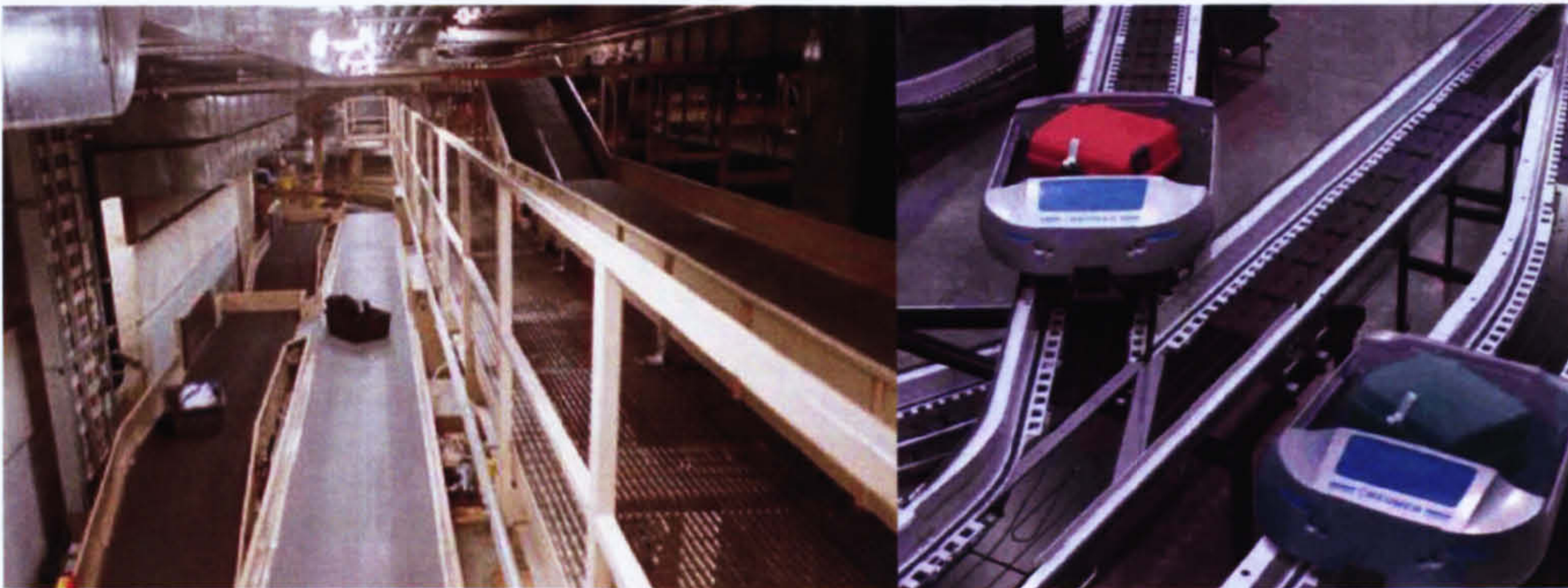
Figure 2.12– Conveyor (left) and DCV (right) networks for transporting baggage
