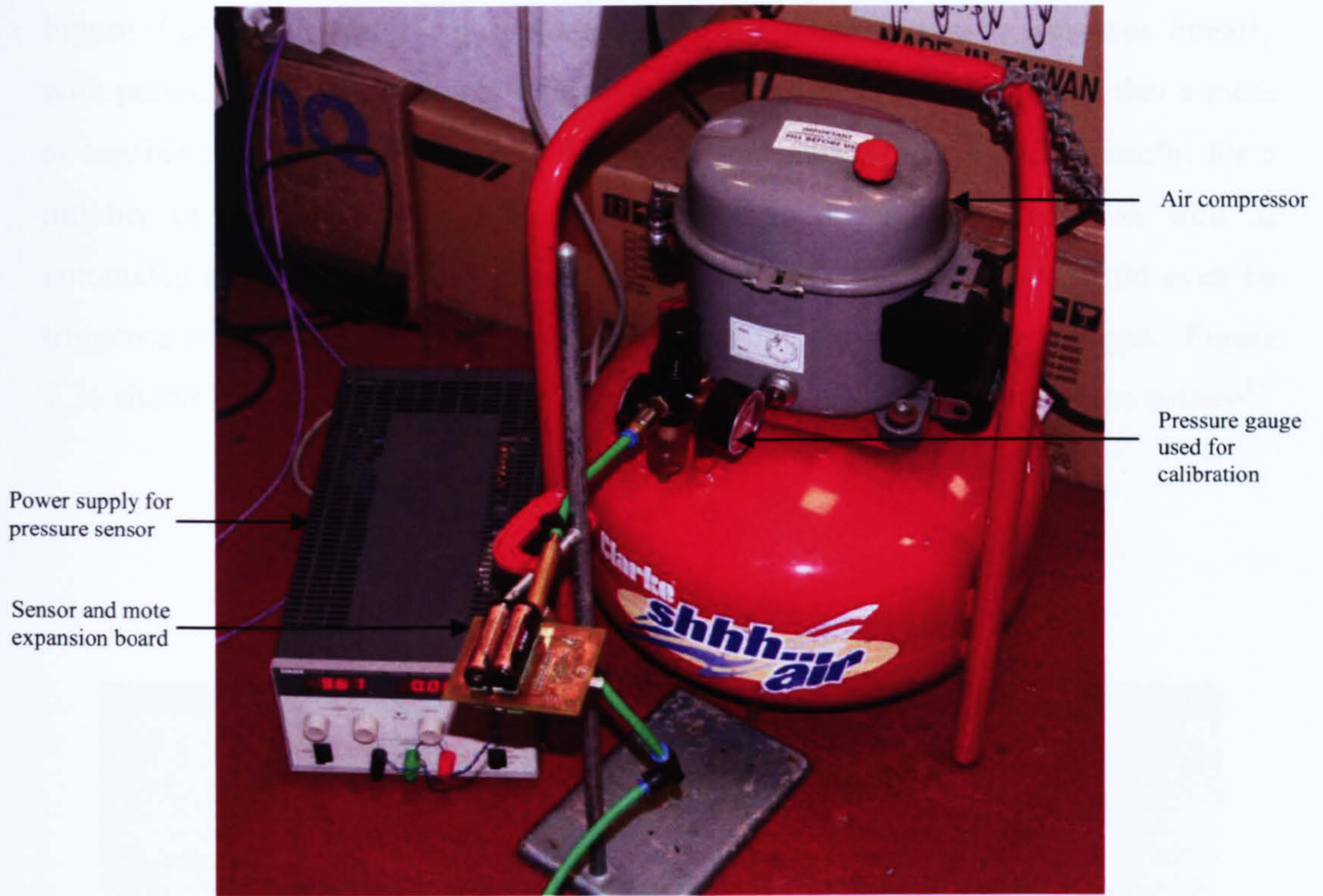
Figure 7.24 – Pressure sensor calibration and test setup
