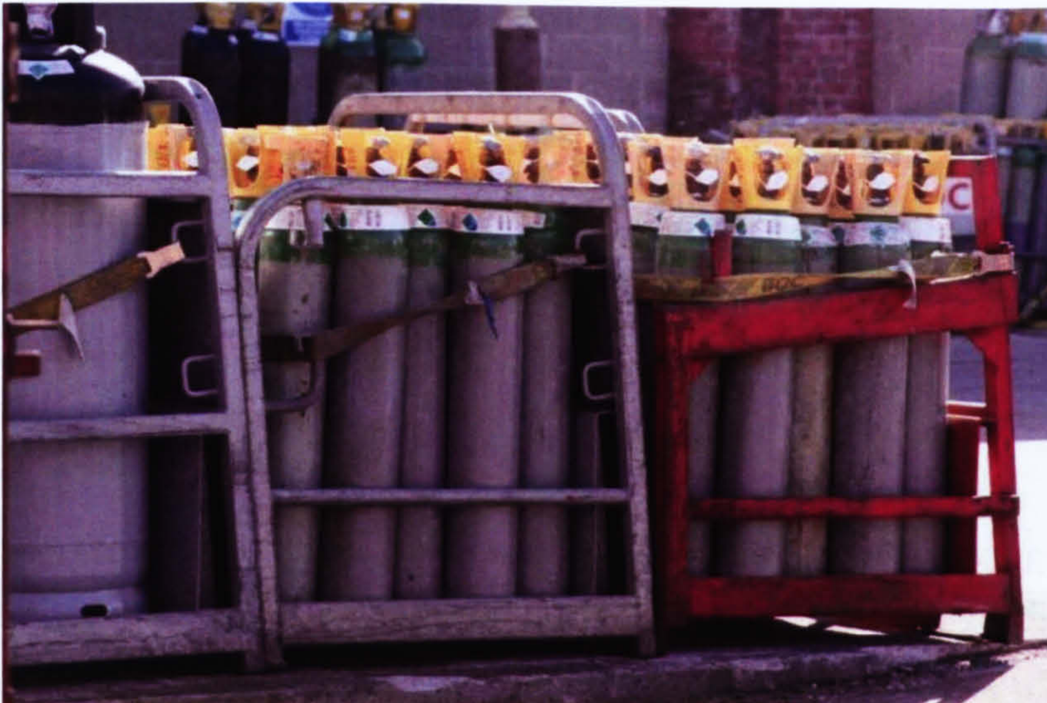
Figure 2.18 – Gas cylinders in storage racks
