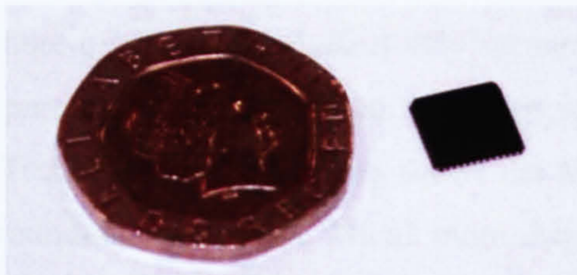
Figure 8.1 – System on chip integrated circuit for future motes
