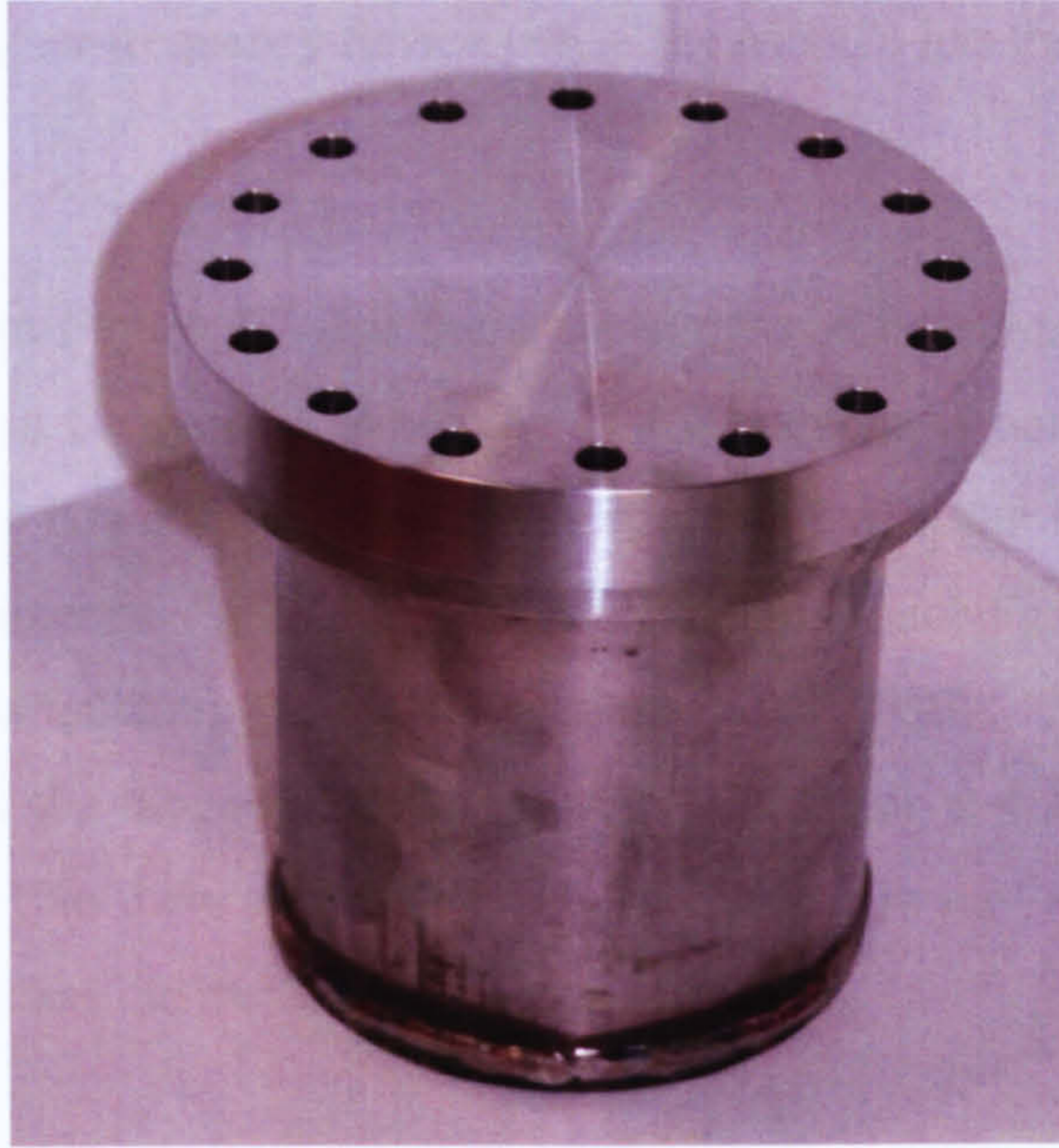
Figure 7.5 – Sealed metal chamber not allowing RF communication
