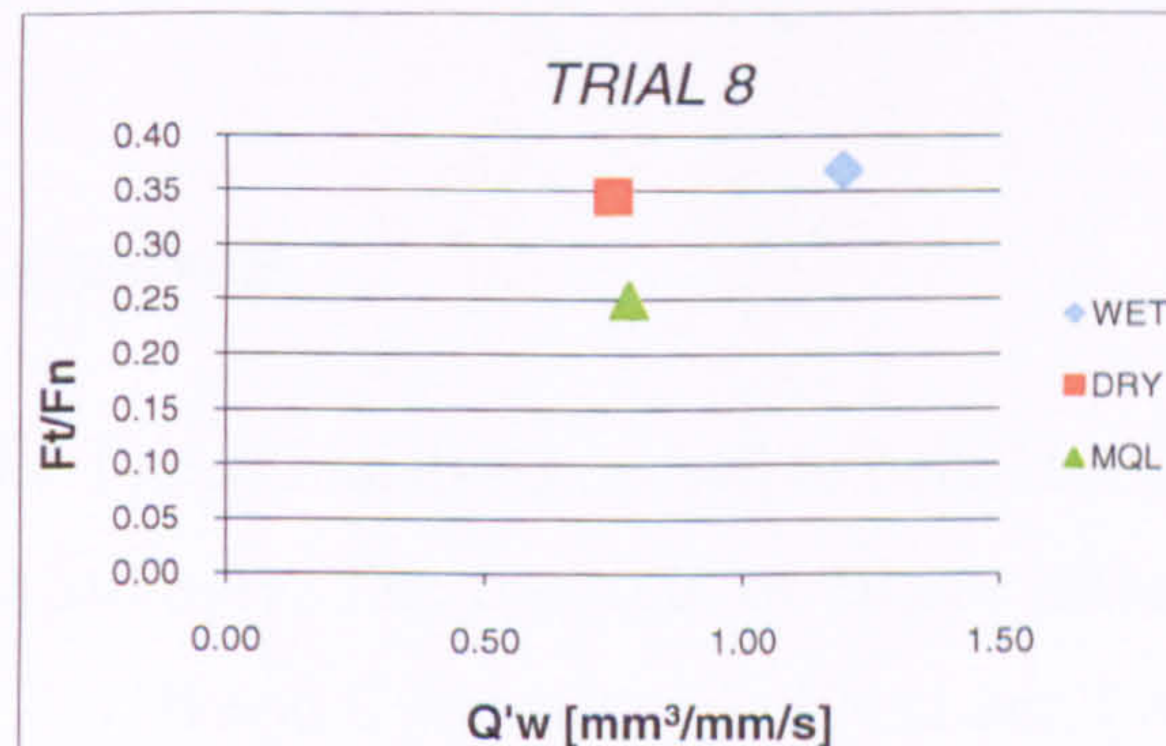
Figure 7-15. Coefficient friction F_t/F_n in function of specific removal rate Q'_w for hard material EN31.
