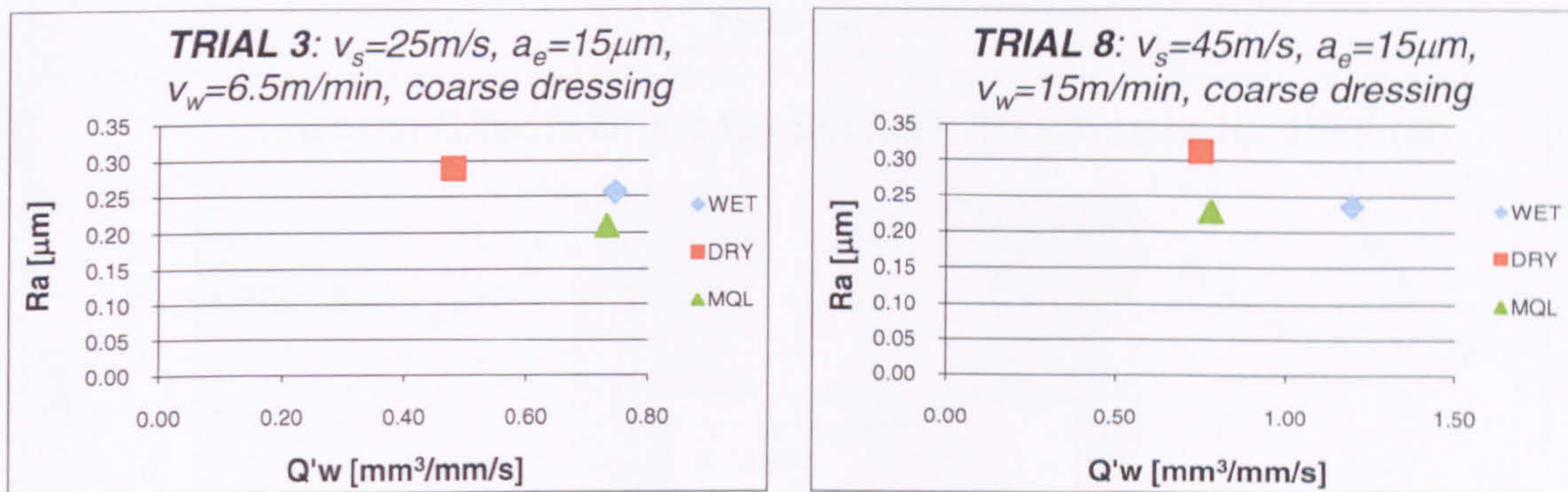
Figure 7-23. Surface roughness R_a in function of specific removal rate Q'_w for hard material M2.
