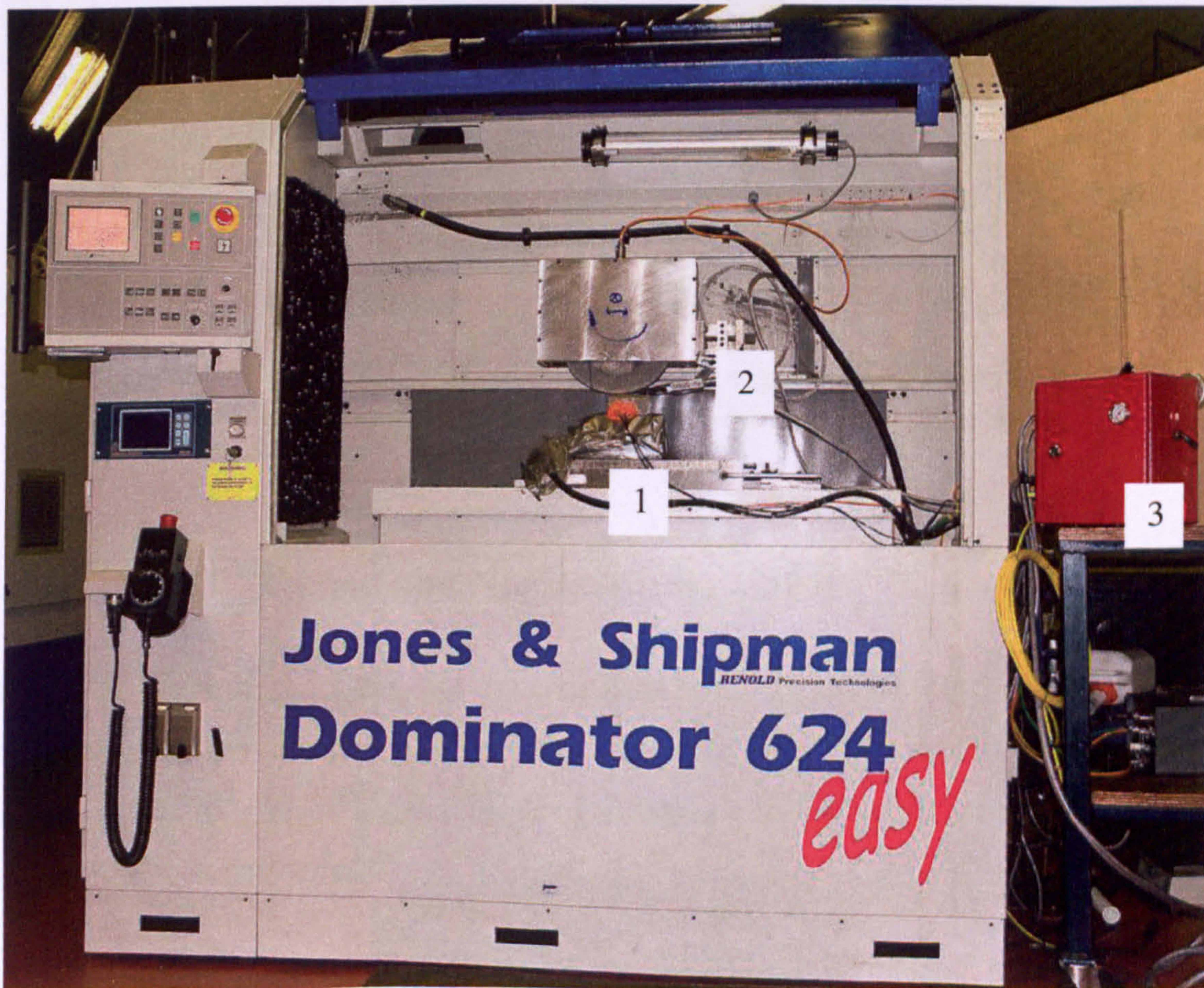
Figure 6-1. CNC Jones&Shipman Dominator 624 Easy with open front hosing: 1 – dynamometer, 2 – nozzle, 3 – MQL system.
