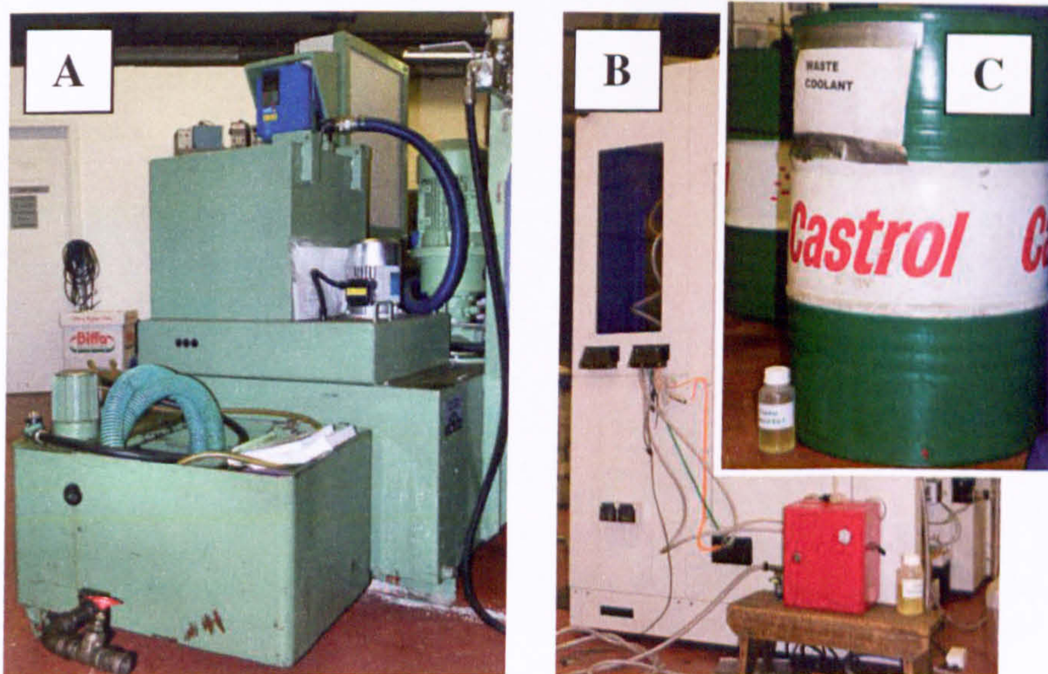
Figure 7-36. Comparison of fluid delivery systems (in scale) – conventional system (A), MLQ system (B) and amounts of fluid used – i.e. bottle compared to barrel (C).
