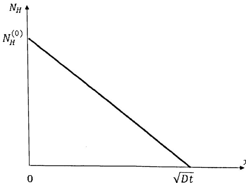
Fig 4.3 Approximate concentration of  $H^0$  in the diffusion process.
