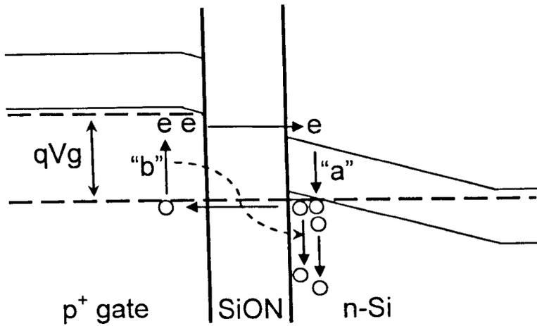
Fig 4.12 A schematic diagram showing the physical processes for generating hot holes under  $V_g = -1.2$  V. The process “a” shows that the energy released by the electron-hole recombination in the substrate can create hot holes. The process “b” shows that the photons emitted from the gate can be absorbed to generate hot holes.
