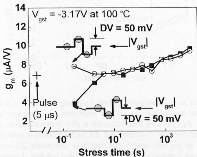
Fig 3.4 The classical transconductance,  $g_m$ , during NBTI test. The symbol '+' was obtained from a pulse ( $5 \mu\text{s}$ )  $I_d \sim V_g$  and should be used as the initial  $g_m$ . The symbol 'o' and '■' were measured by a quasi-DC parameter analyzer and the time for obtaining one  $I_d$  point is 150 ms.
