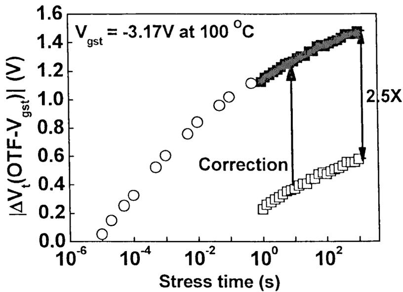
Fig 3.5 Impact of degradation during measurement on  $|\Delta V_t|$ . When the stress time was less than 1 s, the symbol 'o' was obtained by pulse measurements with a measurement time of 5  $\mu$ s. When the stress time was longer than 1 s, the symbol '□' was measured using a quasi-DC parameter analyzer and it took 150 ms to obtain the reference  $I_d$  and this reference  $I_d$  was not degradation free.
