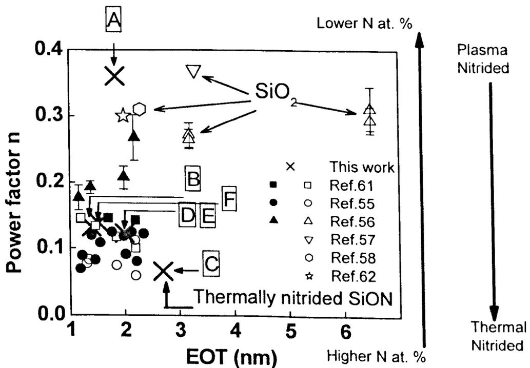
Fig 4.17 A comparison of the power factor obtained in this work with that reported by earlier work.
