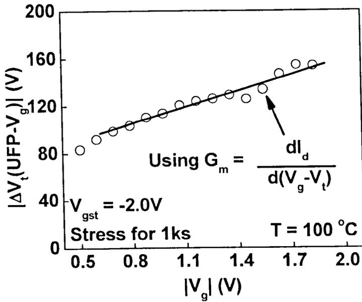
Fig 3.11 Dependence of  $|\Delta V_t|$  on sensing  $V_g$  after stressing at a relatively low  $V_{gst} = -2.0V$  for 1000 s. The  $V_g$  effect is still substantial.
