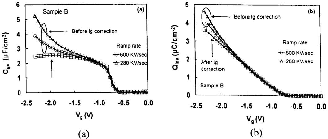
Fig 5.7 (a)  $C_{gc}$  is measured by the pulse C-V technique with 600 kV/s and 280 kV/s ramp rate respectively. The thickness of the device used in the test is 1.13 nm and therefore the leakage current is much more severe than the case shown in fig 5.5.  $C_{gc}$  before and after correction agrees reasonably well within -1.2V and then begin separating. (b) shows the inversion charge integrated by using  $C_{gc}$  before and after correction.
