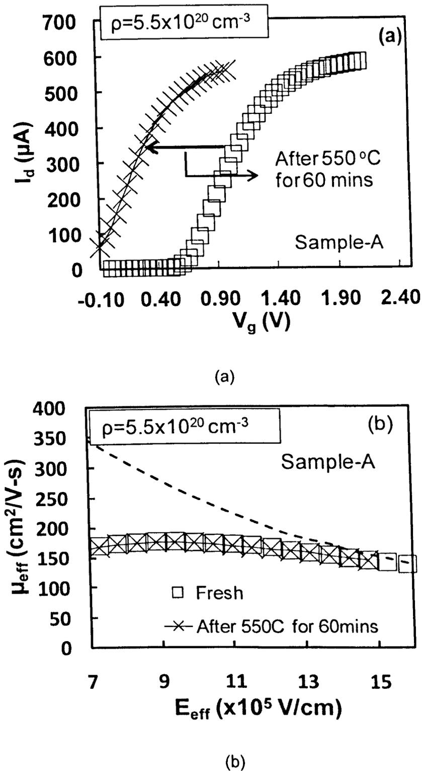
Fig 5.10 The transfer characteristics of sample A before and after a 60 minutes annealing are shown in (a). A positive charging of  $5.5 \times 10^{20} \text{ cm}^{-3}$  is generated in  $\text{HfO}_2$ . The effective electron mobility before and after the 60 minutes annealing is shown in (b). The dash line is the universal curve.
