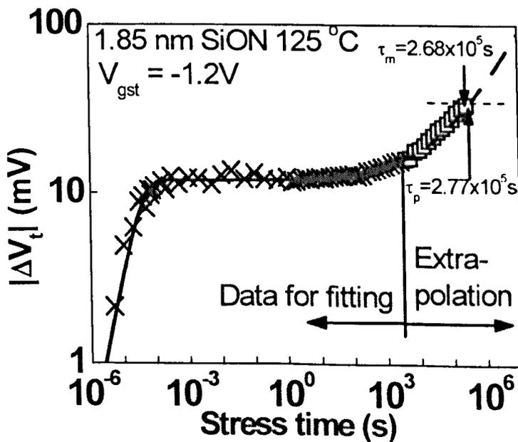
Fig 4.15 Lifetime prediction based on our model: the equation (4.12). The test data is the same as those in Figs. 13 and 14 and only symbol "x" was used for fitting.
