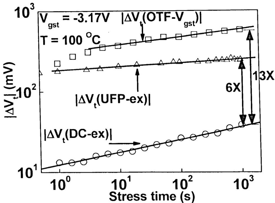
Fig 3.2 Comparison of threshold voltage shift,  $|\Delta V_t|$ , measured by OTF- $V_{gst}$ , UFP-ex and conventional DC-ex technologies.
