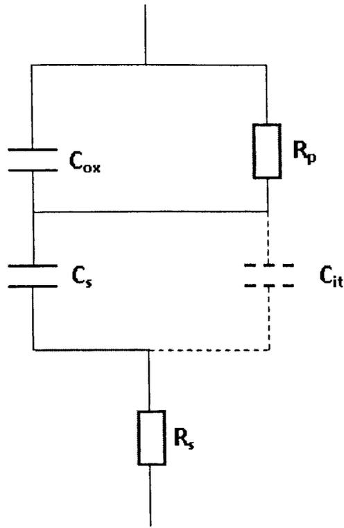
Fig 2.2 Equivalent circuit of an MOS structure.
