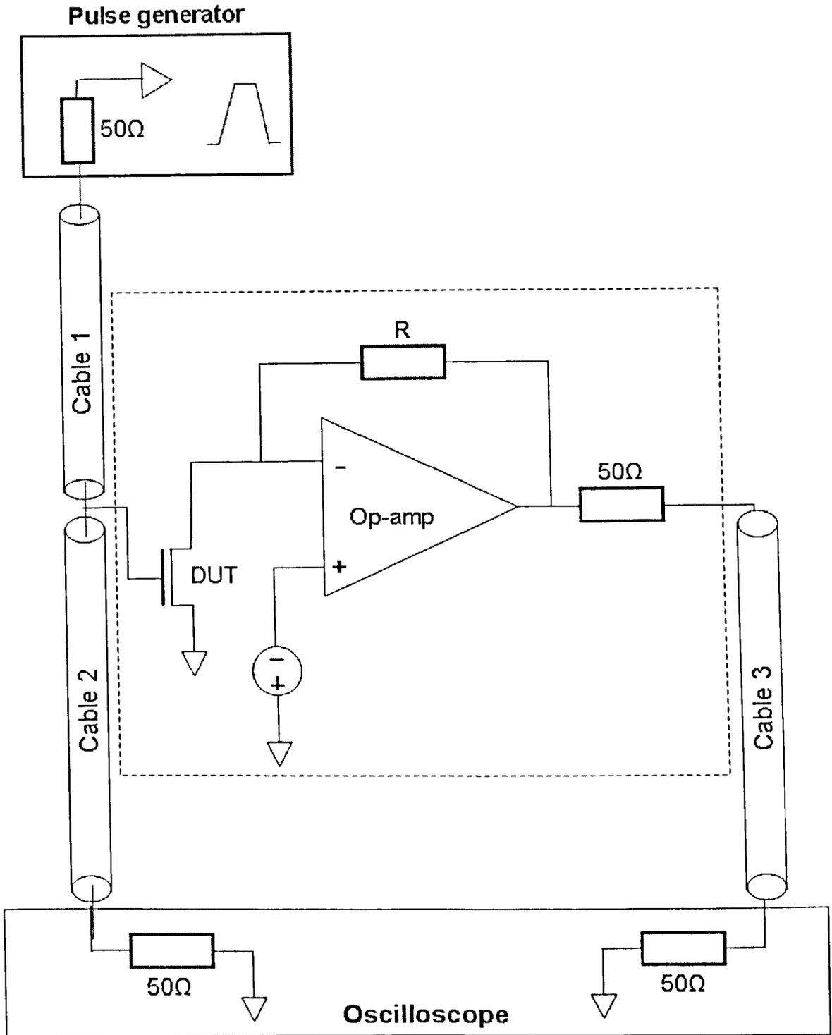
Fig 2.13 Schematic setup for ultra fast pulse measurement by using op-amplifier (AD844) with matched impedance and controlled cable delay.
