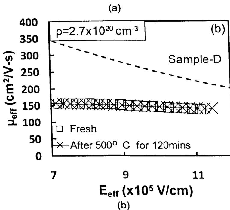
Fig 5.13 The transfer characteristics before and after 120 minutes annealing of the sample D are shown in (a). A PIPC of  $2.7 \times 10^{20} \text{ cm}^{-3}$  was generated. The effective electron mobility before and after the 60 minutes annealing is shown in (b). The dash line is the universal curve.
