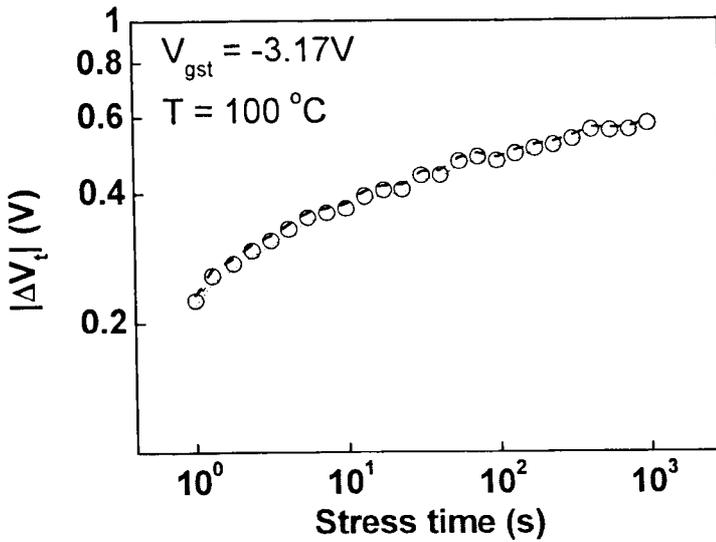
Fig 2.8 The effect of  $g_m$  on  $\Delta V_t$ . Symbol 'O' is calculated using the average  $g_m$  value between two measurement points, while the dashed line used the previous  $g_m$  value, and the dot line uses the current  $g_m$  value. It is clear that  $\Delta V_t$  is weakly dependent on the  $g_m$  value used.
