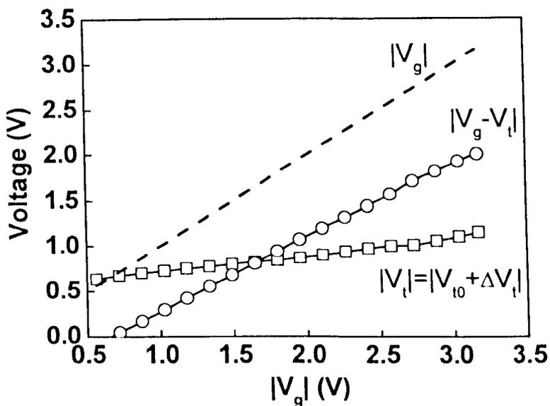
Fig 3.18 The device is stressed at  $-3.17 \text{ V}$  for  $1 \text{ ks}$  under  $100 \text{ }^\circ\text{C}$  condition.  $|\Delta V_t|$  can be as large as  $0.7 \text{ V}$ . Although an increase of  $|\Delta V_t|$  results in an increase of  $|V_t|$  for higher  $|V_g|$ ,  $|V_g - V_t|$  still increases with  $|V_g|$ , so that the MOSFET can be switched on and  $I_d$  increases with  $|V_g|$ .
