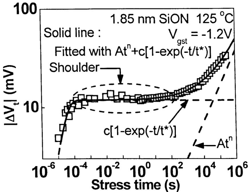
Fig 4.8 The kinetic feature of the UFP  $\Delta V_t$  sensed at  $|V_g|=1.2$  V: a “shoulder”. By combining the 1<sup>st</sup> order model for as-grown hole traps with the power law for defect generation,  $\Delta V_t$  can be fitted over 10 orders of magnitude in time, as shown by the solid line. The dashed lines show that  $\Delta V_t$  is dominated by as-grown hole traps initially, but the generated defects become important at longer stress time.
