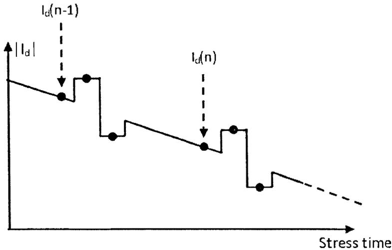
Fig 2.7 The  $n^{\text{th}}$  and  $n-1^{\text{th}}$   $I_d$  measurements, together with the transconductance  $g_m(n)$ , can give the threshold voltage shift,  $\Delta V_t$ , between  $n^{\text{th}}$  and  $n-1^{\text{th}}$  measurement points.
