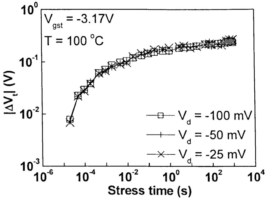
Fig 2.17 Effect of drain voltage on the NBTI degradation. Drain voltage up to 100mV will not affect the experimental result.
