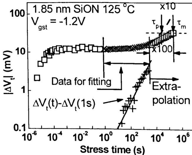
Fig 4.14 Lifetime prediction based on the method proposed in [53]. All symbols are test data but only symbol “x” was used for fitting.  $\Delta V_t(t) - \Delta V_t(1\text{ s})$  (the symbol “+”) was fitted with a power law and  $\Delta V_t(1\text{ s})$  was then added back. The dashed line is extrapolated for prediction.  $\tau_m$  is the time for the last test point and  $\tau_p$  is the predicted time.
