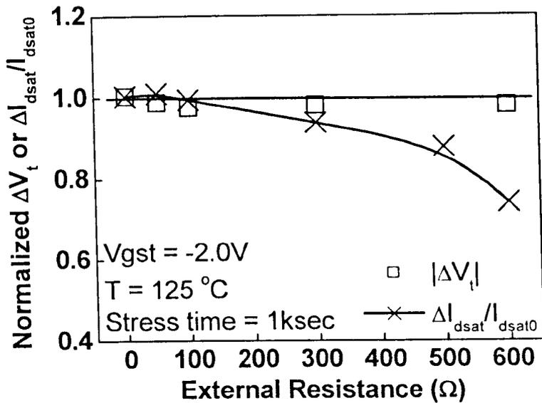
Fig 3.26 Dependence of  $\Delta I_{dsat}/I_{dsat0}$  and  $|\Delta V_t|$  on the series resistance. The 'external resistance',  $R_{ext}$ , is a resistor externally connected to the drain of the devices under test. Both  $\Delta I_{dsat}/I_{dsat0}$  and  $|\Delta V_t|$  were normalized to their value at  $R_{ext}=0$ .
