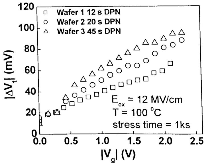
Fig 3.12 Insensitivity of the  $V_g$  effect to fabrication processes. The samples used here are nitrided by DPN with different nitridation time, leading to a different nitridation concentration.
