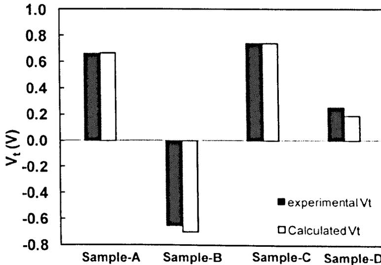
Fig 5.15 A comparison of the measured threshold voltage for fresh devices with their theoretical values. The theoretical value is calculated by using equation (5.26). The experimental value is extracted by using constant current method at the level of  $1 \times 10^{-6} \text{W/L}$ .
