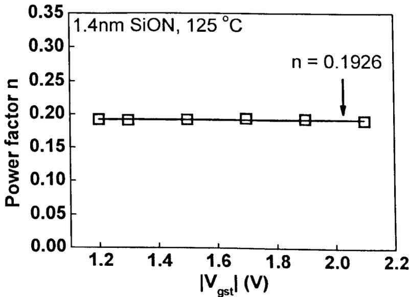
Fig 4.6 The power factor  $n$  from DC-ex measurement. It is insensitive to the stress bias. The solid line represents the average power factor of  $n=0.1926$ .
