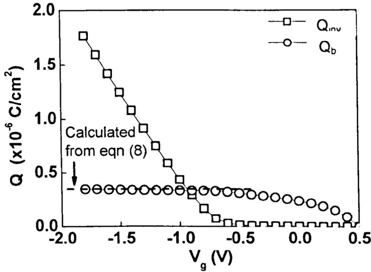
Fig 5.6 Inversion charge  $Q_{inv}$  and bulk charge density  $Q_b$  obtained from equation (5.5) and equation (5.6).  $Q_b$  calculated from equation (5.8) is represented by the dashed line. The substrate doping in our sample is  $5 \times 10^{17} \text{ cm}^{-3}$ .
