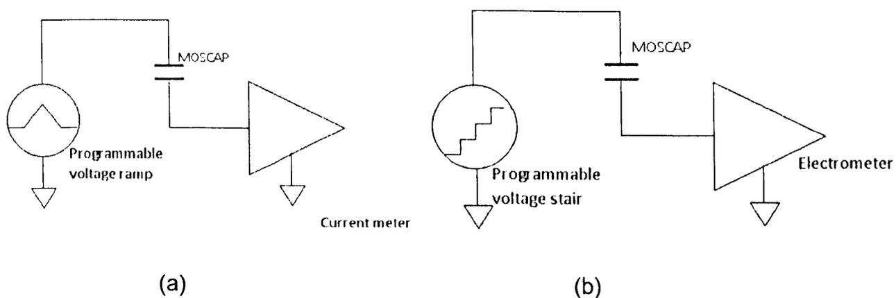
Fig 2.5 (a) Schematic configuration of quasi-static measurement setup using a linear voltage ramp; (b) schematic configuration of equilibrium controlled quasi static measurement setup where discrete voltage steps are applied and the displacement charge is measured using an electrometer.
