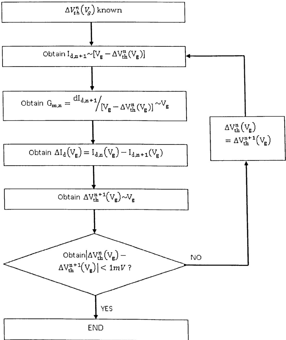
Fig 3.9 Flow chart of the  $|\Delta V_t|$  evaluation by iteration.
