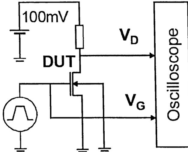
Fig 2.9 Schematic setup for the pulse  $I_d$ - $V_g$  measurement proposed by A.Kerber et al. The MOSFET was used in an inverter circuit with a resistive load ( $R$ ). From the voltage waveform ( $V_g(t)$ ,  $V_d(t)$ ), the  $I_d$ - $V_g$  characteristics were extracted.
