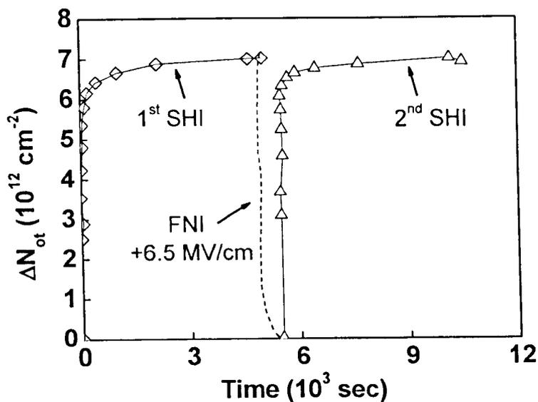
Fig 3.17 Positive charging during substrate hole injection (SHI). The charging density can be routinely over  $6 \times 10^{12} \text{ cm}^{-2}$ . The figure is taken from [17].
