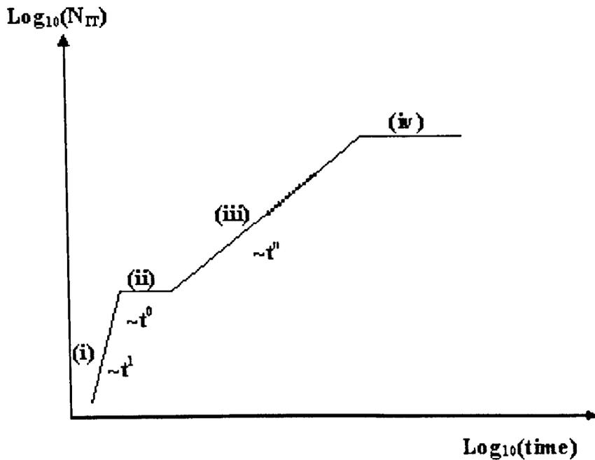
Fig 4.2 Schematic time evolution of the classic R-D model. Regions: (i) generation-limited, (ii) dynamic equilibrium, (iii) diffusion-limited, and (iv) saturation. Region (iii) gives the power-law behaviour for NBTI.
