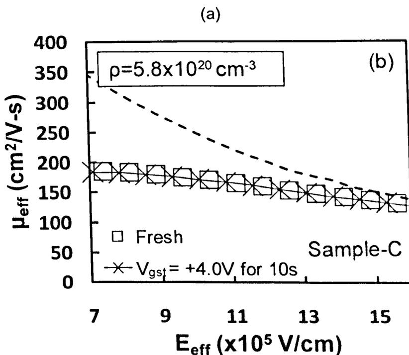
Fig 5.12 The sample C was stressed at +4.0V for 10 s and an electron trapping of  $5.8 \times 10^{20} \text{ cm}^{-3}$  are formed. The transfer characteristics before and after electron trapping are shown in (a). The effective electron mobility before and after electron trapping is shown in (b). The dash line is the universal curve.
