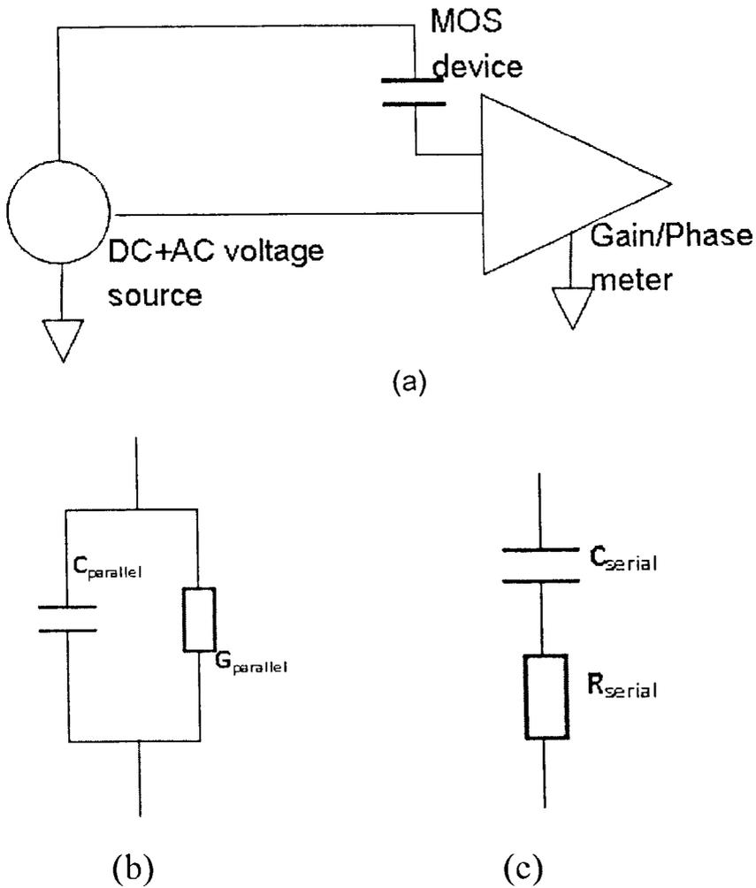
Fig 2.3 (a) Schematic configuration of high frequency C-V measurement. The DC and AC bias is applied to one terminal of the capacitor whereas the gain and phase of the AC signal is measured on the second terminal. (b) Equivalent circuit of a HF C-V taken in the parallel mode, (c) Equivalent circuit of a HF C-V taken in a serial mode
