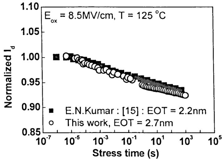
Fig 3.7 Drain current degradation comparison of the result with that of Kumar et al [15]
