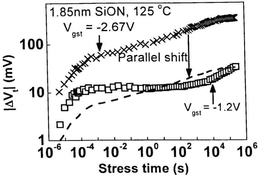
Fig 4.7 The kinetics at different  $V_{gst}$  is not shifted in parallel for the UFP  $\Delta V_t$  sensed at  $|V_{gl}|=1.2$  V. The dashed curve was obtained by shifting the symbol 'x' downward in parallel.
