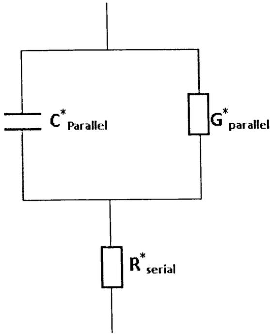
Fig 2.4 Simplified equivalent circuit of a MOS device with parallel conductance and serial resistance.
