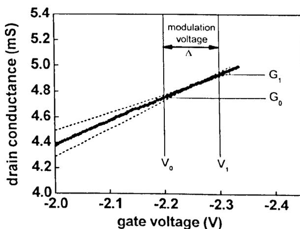
Fig 3.13 Figure from Reisinger et al work [16]. The dashed straight lines illustrate how even a small change in conductance at stress level leads to a large variation at the lower  $V_g$  where the threshold voltage is evaluated.
