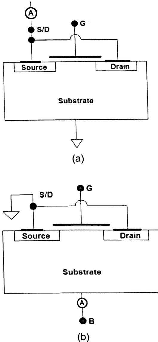
Fig 5.1 Configuration for split C-V technique. Conventionally, split C-V technique is performed by using LCR meters. (a) In order to measure gate-to-channel capacitance,  $C_{gc}$ , the terminal marked HI is connected to the gate and LO to the source and drain, the substrate of the device is connected to GND. (b) In order to measure gate-to-substrate capacitance,  $C_{gb}$ , the terminal HI is connected to the gate and LO to the substrate.
