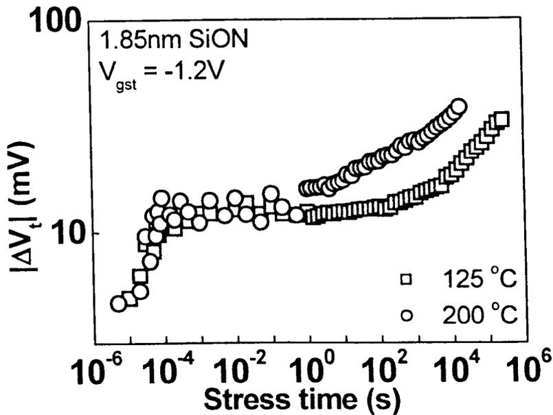
Fig 4.9 Effect of temperature on NBTI kinetics. The height of the shoulder is insensitive to temperature, but the generation of defects above the shoulder is thermally accelerated.
