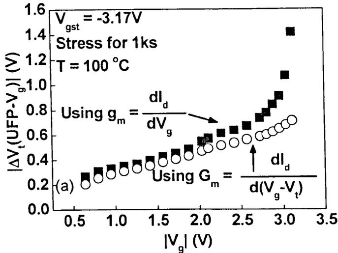
Fig 3.10 Impact of transconductance evaluation on the accumulative  $|\Delta V_t|$ . The sample is stressed at  $-3.17V$  for 1000 s. When the classical  $g_m = dI_d/dV_g$  was used,  $|\Delta V_t|$  was substantially overestimated at high sensing  $|V_g|$ .
