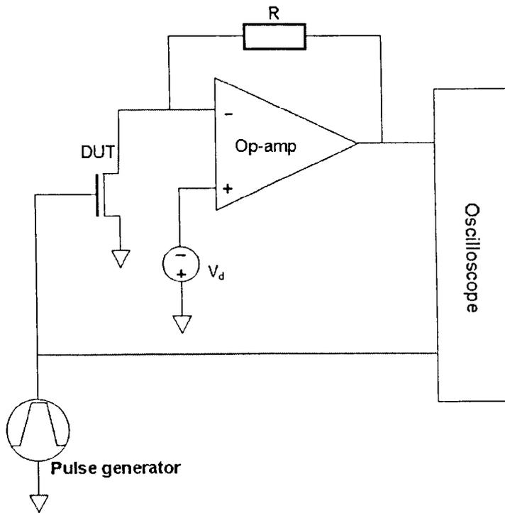
Fig 2.11 Schematic setup for the ultra fast pulse  $I_d$ - $V_g$  technique
