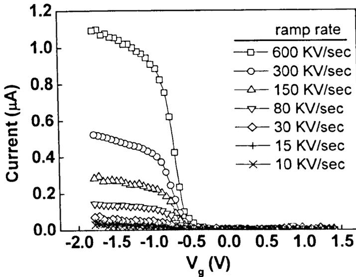
Fig 5.3 Displacement current measured from the MOSFET with an EOT of 1.53 nm and a typical area of  $100 \mu\text{m}^2$ . The magnitude of the displacement current drops for lower ramp rate. When ramp rate is lower than 30 kV/s, the displacement current is below  $10^{-8}$  A and it is not easy to measure accurately.
