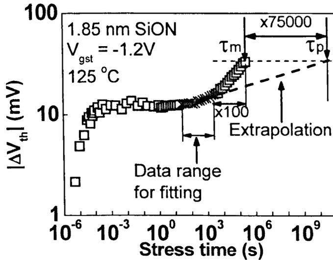
Fig 4.13 Lifetime prediction based on the method proposed in ref. 5. All symbols are test data but only symbol “x” was used for fitting with a power law in the range of 26.8 s < t < 2680 s. The thick dashed line is extrapolated from the fitted line for prediction.  $\tau_m$  is the time for the last test point and  $\tau_p$  is the predicted time.
