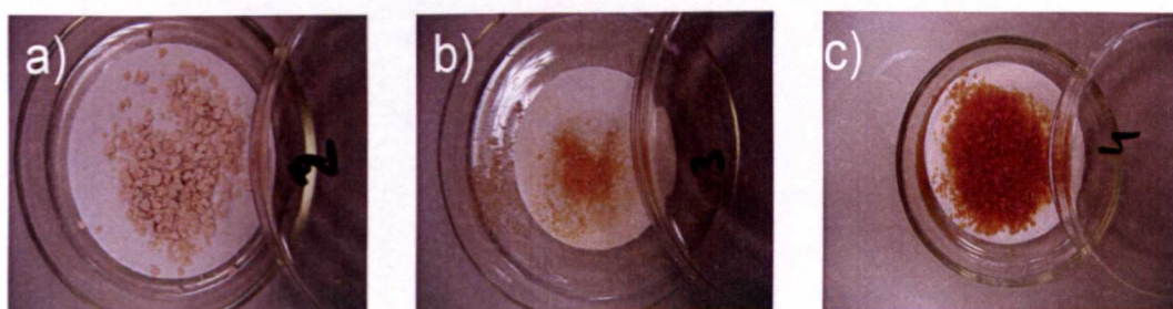
Figure 2.5: Effect of volume of anhydrous THF on enzyme support integrity after 24hours: (a) 20 ml, (b) 10 ml and (c) 5 ml.
