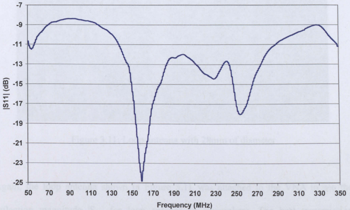
Figure 3.10: Reflection magnitude |S_{11}| for monopole antenna in water
