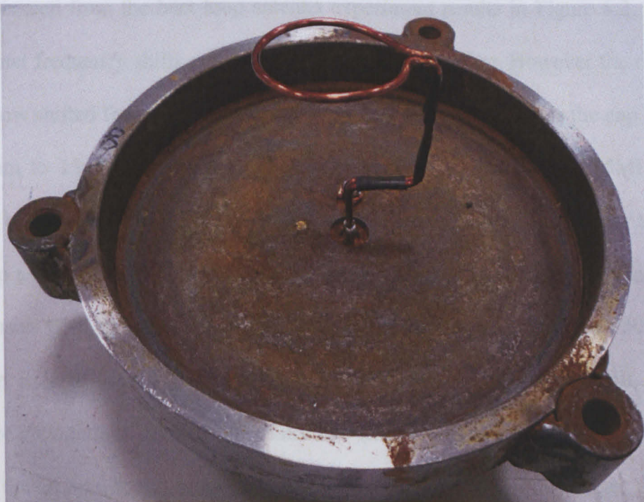
Figure 6.1: Loop antenna bent to 90 degrees from the axis of the pipe to fit with Balfour Beatty's requirements
