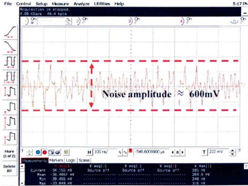
Fig.2.13. After the improvement, system noises were reduced to 600mV.
