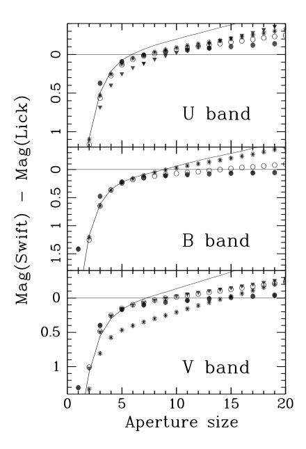
Fig. 7.— The difference between the UVOT photometry and the Lick calibrations, as a function of aperture size. The same symbols have been used as in Figure 6.
