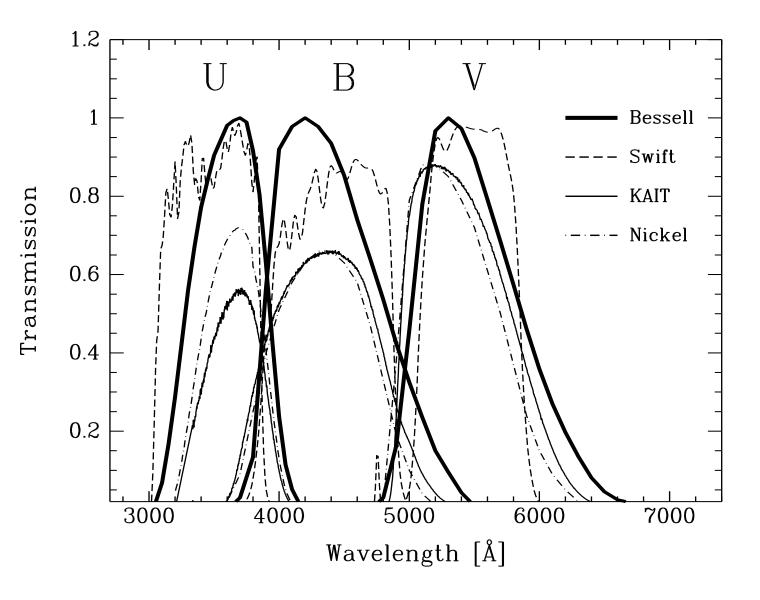
Fig. 3.— The U, B, and V filter transmission curves. Plotted are the filters used by KAIT (thin solid lines), Nickel (dash-dotted lines), and UVOT (dashed lines). The Bessell (1990) descriptions are plotted as thick solid lines.
