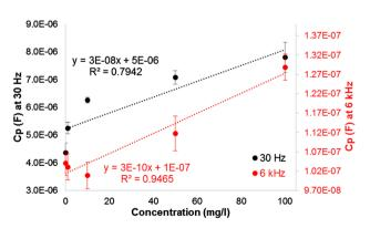
Fig. 5 Correlation between capacitance (measured with a LCR meter) and metal concentration at two discrete frequencies: 30 Hz and 6 kHz
