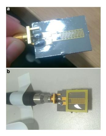
Fig. 2 a Eight-pair IDE sensor with PCB lacquer coating and SMA connector; **b** sensor with a tested sample of lead-contaminated water solution deposited onto the sensor and kept in place with an adhesive FR4 well holder
