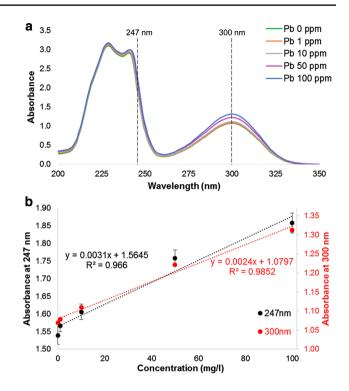
**Fig. 4 a** Average absorbance spectrum of various lead solutions in 200–350 nm range measured with a UV–Vis spectrophotometer; **b** linear correlations for the absorbance with concentration of lead at two wavelengths, namely 247 and 300 nm
