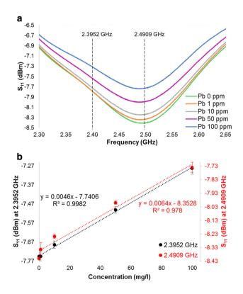
**Fig. 10 a** Part of average microwave spectra of lead solutions in the frequency range 2.3-2.65 GHz; **b** two specific frequencies are evidenced, namely 2.3952 and 2.4909 GHz (peak), demonstrating linear correlations between reflected power (S<sub>11</sub>) and lead concentration
