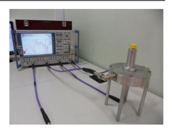
Fig. 1 A laboratory-based electromagnetic wave sensing system comprising the Vector Network Analyser (left) and a bespoke resonant cavity structure (right)
