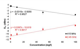
Fig. 8 Change in reflected power  $S_{11}$  of a microwave spectra measured with resonant cavity showing the correlation with metal concentration at two discrete frequencies, namely 415 MHz and 2.45 GHz
