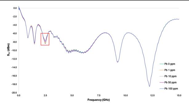
**Fig.9** Average microwave spectra data captured with a gold eightpair IDE sensor at 0.01–15 GHz frequency range for each sample concentration of lead. The red rectangle shows the frequency range
