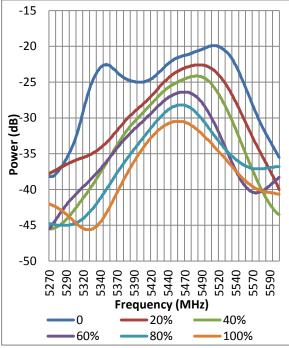
Figure 3. Experimental results from the cylindrical resonant cavity sensor for various fraction of water percentage.
