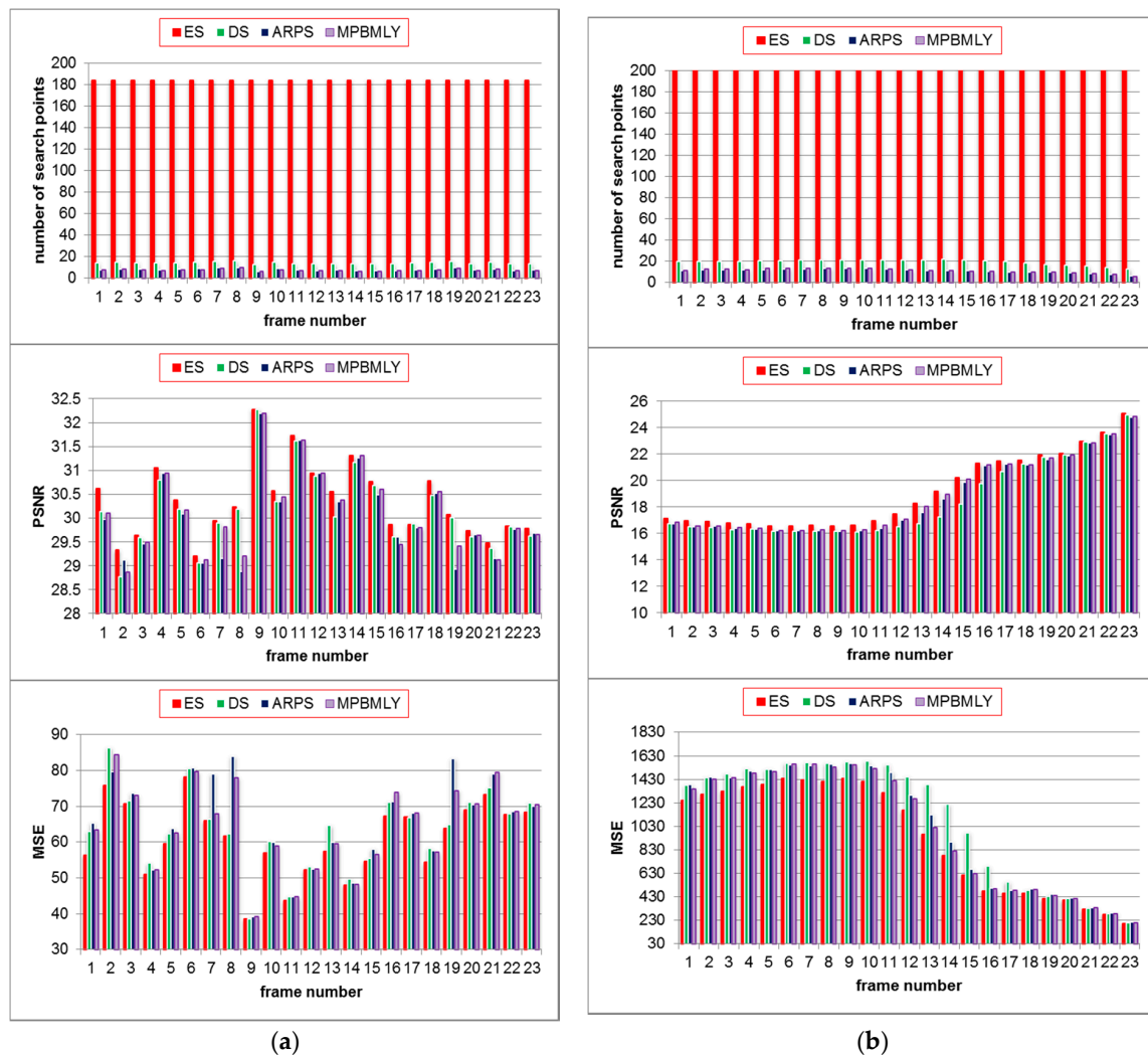
Figure 9. Average number of search points per MB (Top), PSNR performance (Middle), and MSE (Bottom) for MPBMLY and state-of-the-art fast block matching. (a) Average for the “Carphone” video sequence over 23 frames; (b) average for Stefan” video sequence over 23 frames.
