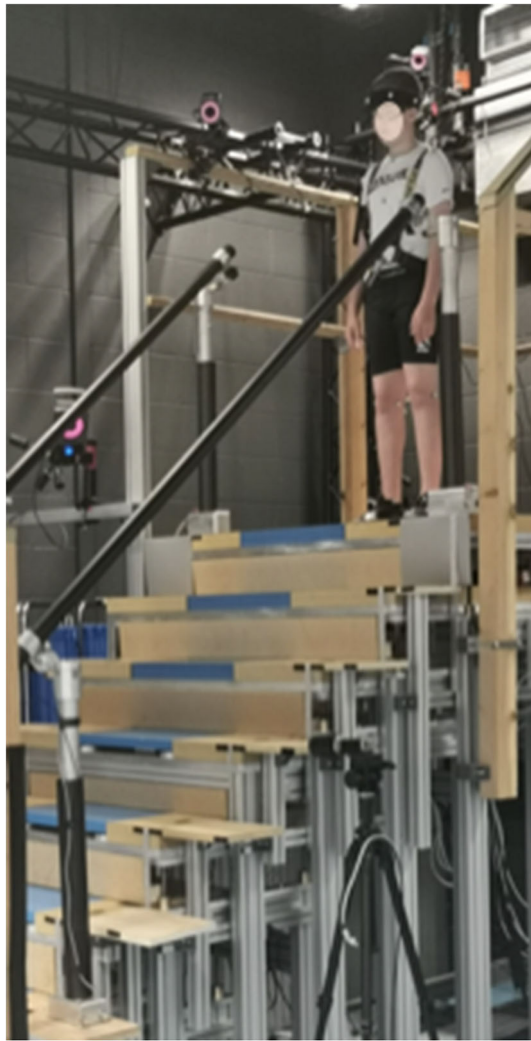
FIGURE 1 | Image displaying a child participant (face blurred) preparing to descend our custom-built instrumented seven-step staircase. The child can be seen wearing a safety harness that is attached to an overhead belay safety system. Each child was allowed to freely use the handrails that can be seen either side of the staircase. The Vicon cameras can also be seen, positioned around the staircase to optimize kinematic data capture.
