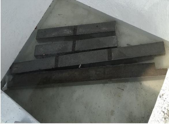
**Figure 21.** Curing of concrete elements
