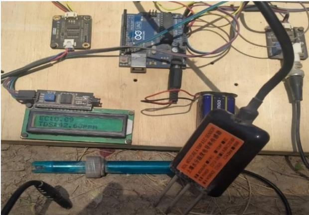
**Fig. 5** Sensor node prototype with sampling in the field
