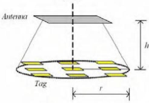
Fig 3 Recognition area model of RFID antenna.
