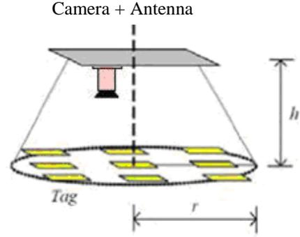
**Fig 8** Recognition area of camera and RFID reader
