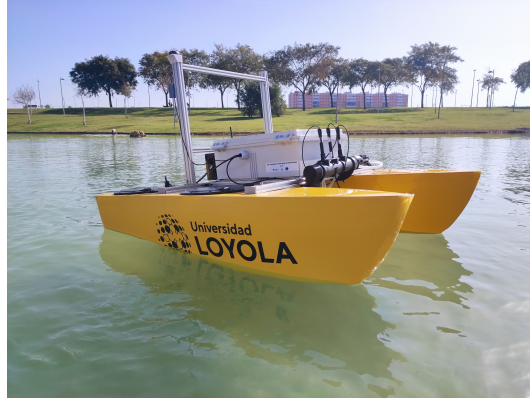
Fig. 1: An Autonomous Surface Vehicle used for the water resource monitoring
