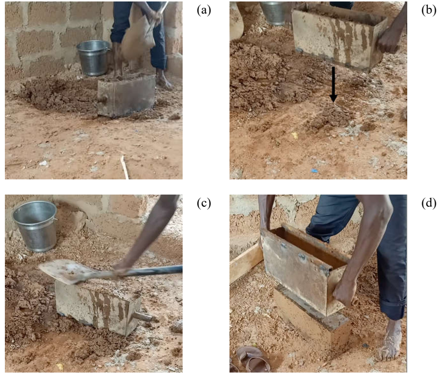
Fig. 4. Brick manufacturing process in Wa: a) filling the mould; b) tamping the mould to achieve the desired density; c) levelling the top of the mould; d) flipping the mould to remove the finished brick
