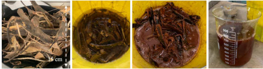
Fig. 2. Processing dawadawa husks. From left to right: the intact husks; the husks soaking in water; the husks after 72 hours (about three days); the extracted solution.
