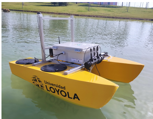
Figure 1: An Autonomous Surface Vehicle used for water resources monitoring.
