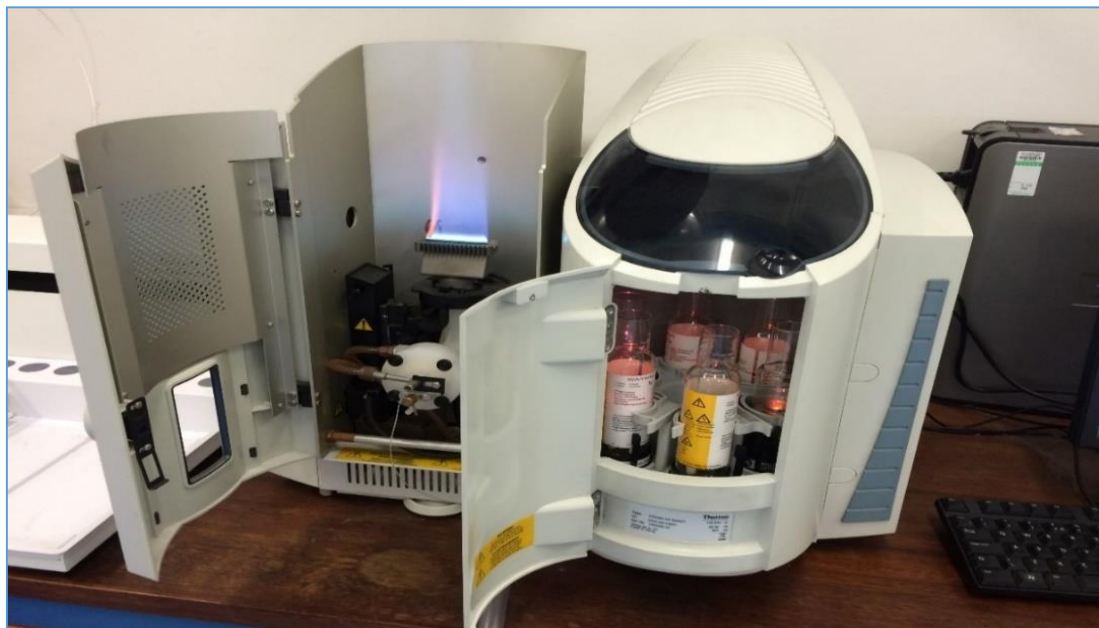
Fig. 3. sample under test using Atomic Adsorption Spectrophotometer.
