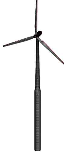
Fig.7 Mesh distribution of single Spar
