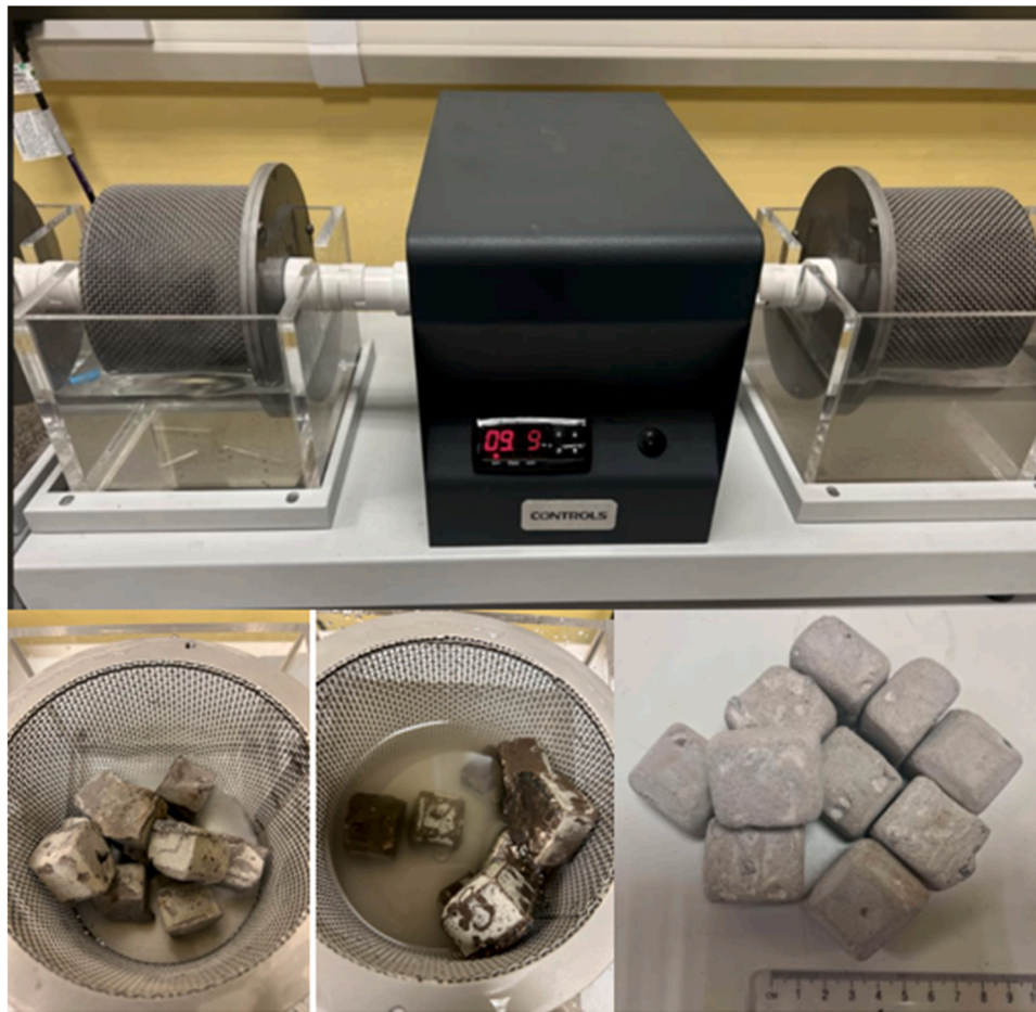
Fig. 2. Experimental setup for the slake durability test.
