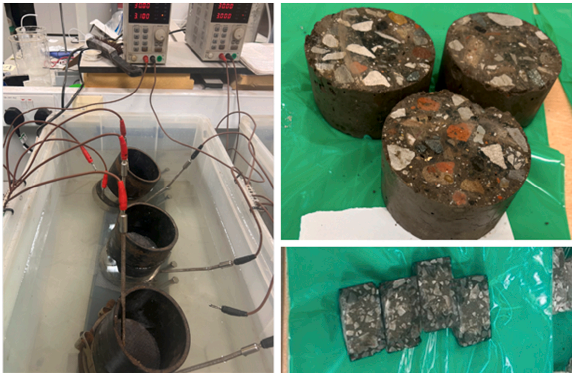
Fig. 3. Chloride migration test set up for the cylindrical samples and bisected samples.
