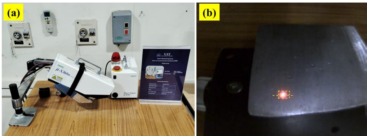
Figure 2. (a) Pulstec \mu -X360n, a portable X-ray residual stress analyzer; (b) X-ray beam on the surface of the graphene-reinforced AA2195 composite sample.
