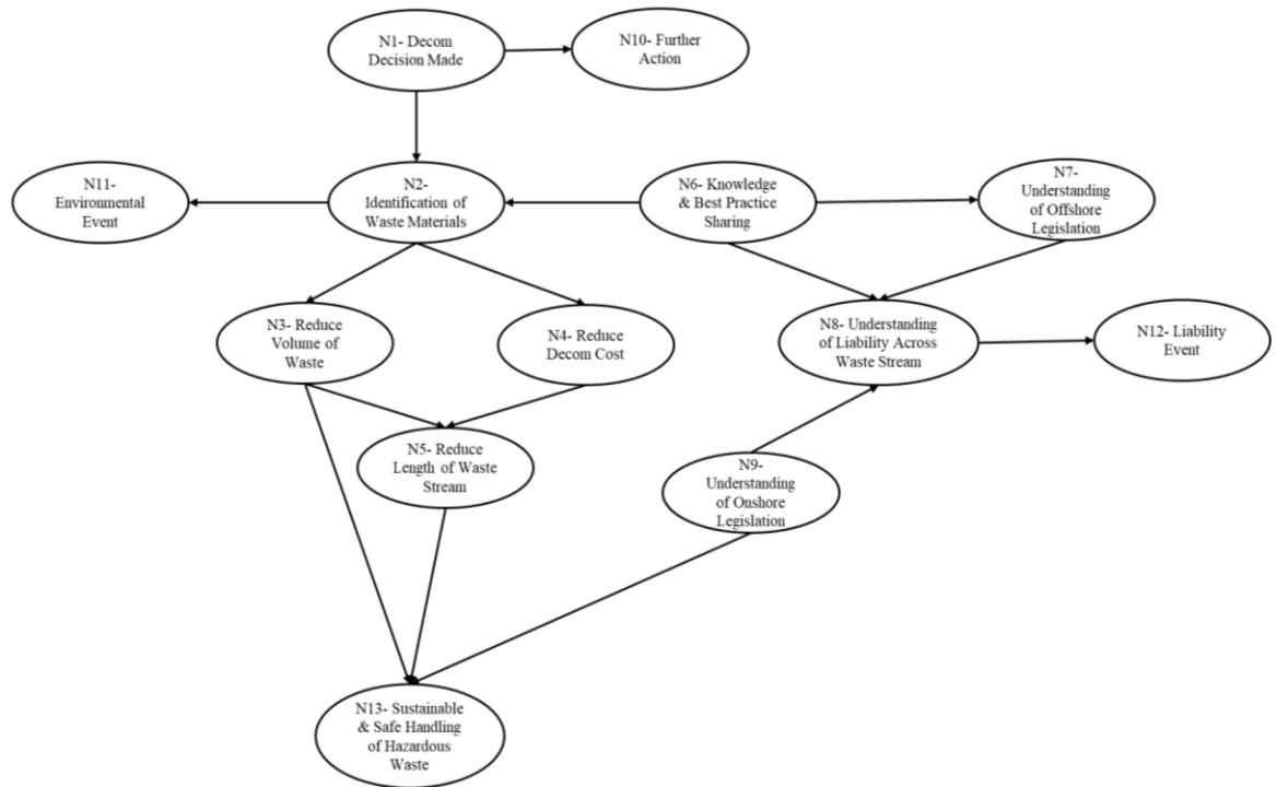
Figure 5-2: Initial BN model illustrating the key factors in the decommissioning process.
