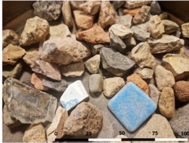
Figure 2: Presence of different types of materials in recycled coarse aggregates (scale in mm)
