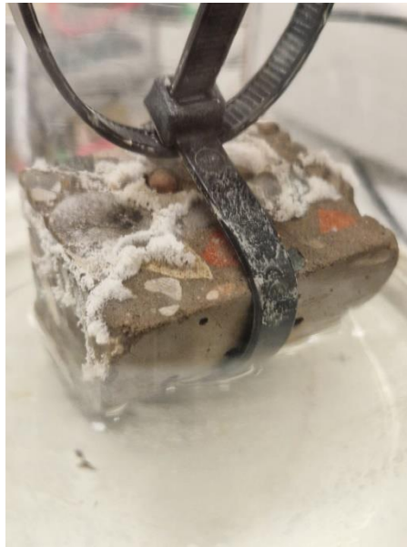
4 5 Figure 12: Appearance of efflorescence on geopolymer samples containing RA
