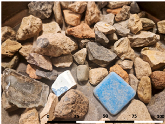
Fig. 2. Presence of different types of materials in recycled coarse aggregates (scale in mm).
