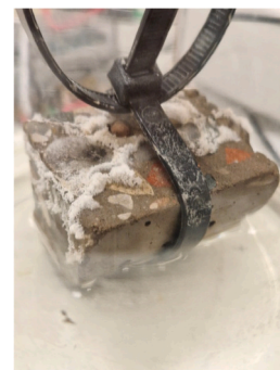
Fig. 12. Appearance of efflorescence on geopolymer samples containing RA.
