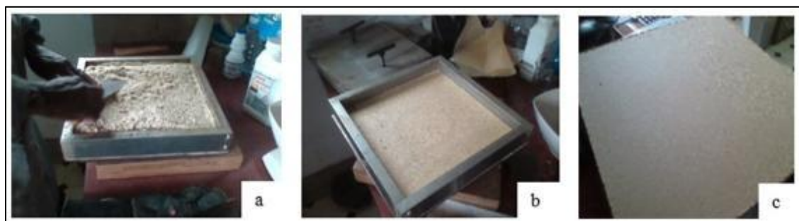
Figure 2 Thermal pressing process: a) Fibers in the mould before thermal pressing, b) the mould out of the pressing machine and c) Demolded fiberboard.
