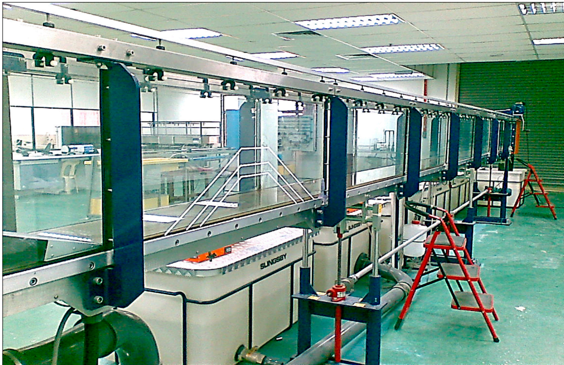
Figure 15. Hydraulic flume with the wave generator.
