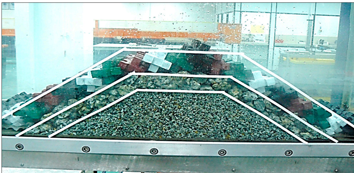
Figure 14. Cross-section of the theoretical structure with a layer of uniformly placed newly designed units (first orientation).
