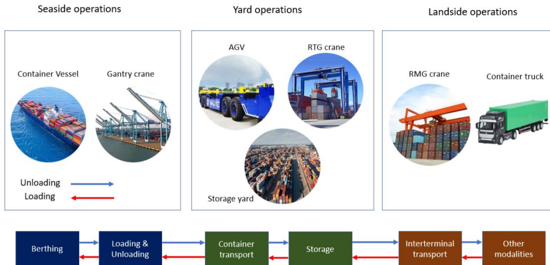
Figure 6. 3: A typical container terminal configuration.
