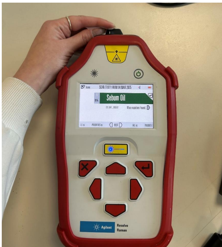
Figure 4.1. The Agilent Resolve Raman spectrometer, equipped with an 830 nm laser wavelength.
