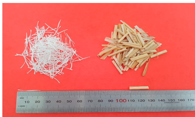
Figure 4. Natural and synthetic fibers used in this study: (left) polypropylene fibers (PPF) and (right) wheat straw fibers (WSF).
