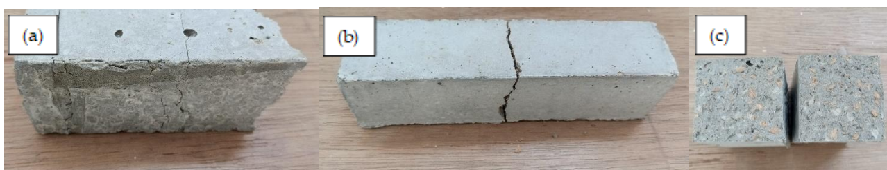
Figure 10. Fracture morphology of specimens after mechanical testing: (a) compressive failure surfaces; (b) flexural failure zones; (c) lateral internal view highlighting porosity and material structure.
