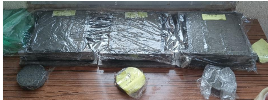
Figure 4. Bio-concrete specimens with 0%, 10%, and 20% olive husk content cast in different molds immediately after mixing.
