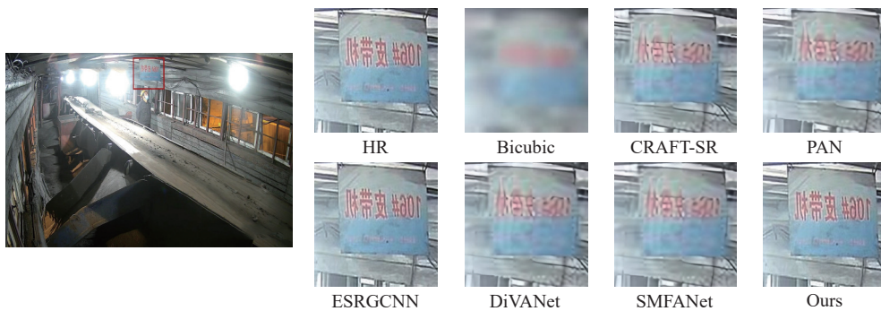
图 12 带式输送机指示牌在缩放因子为 4 倍时的重建效果对比 Fig.12 Comparison of reconstruction effects for belt conveyor signage under 4× scaling
