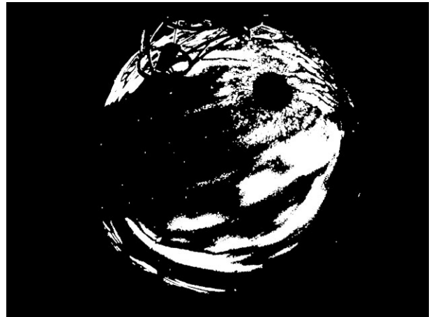
Figure 3. Binary image obtained after the application of the morphology methods (1) erosion and (2) dilation with a 3 \times 3 filter kernel. The number of star pixels is reduced whilst the cloud structure remains intact. Larger filter kernels (e.g. 5 \times 5 or 7 \times 7 ) will remove all stars but also small cloud structures like the ones present in the middle of the image.
