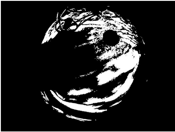
Figure 4. Binary image obtained after an additional star removal step, a simple heuristic is applied to a 21 \times 21 pixel window moved over the whole image, again leveraging fast GPU hardware, to test for small star-shaped pixel areas.
