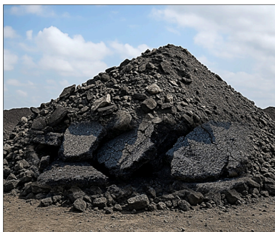
Figure 6. RAP stockpile before homogenization.
