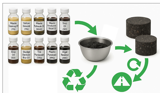
Figure 1. Waste oil rejuvenation process in recycled HMA.
