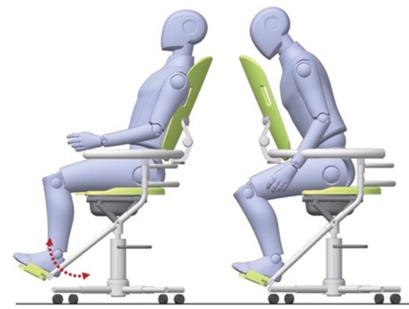
Figure 17. Rotatable Backrest and Footrest
