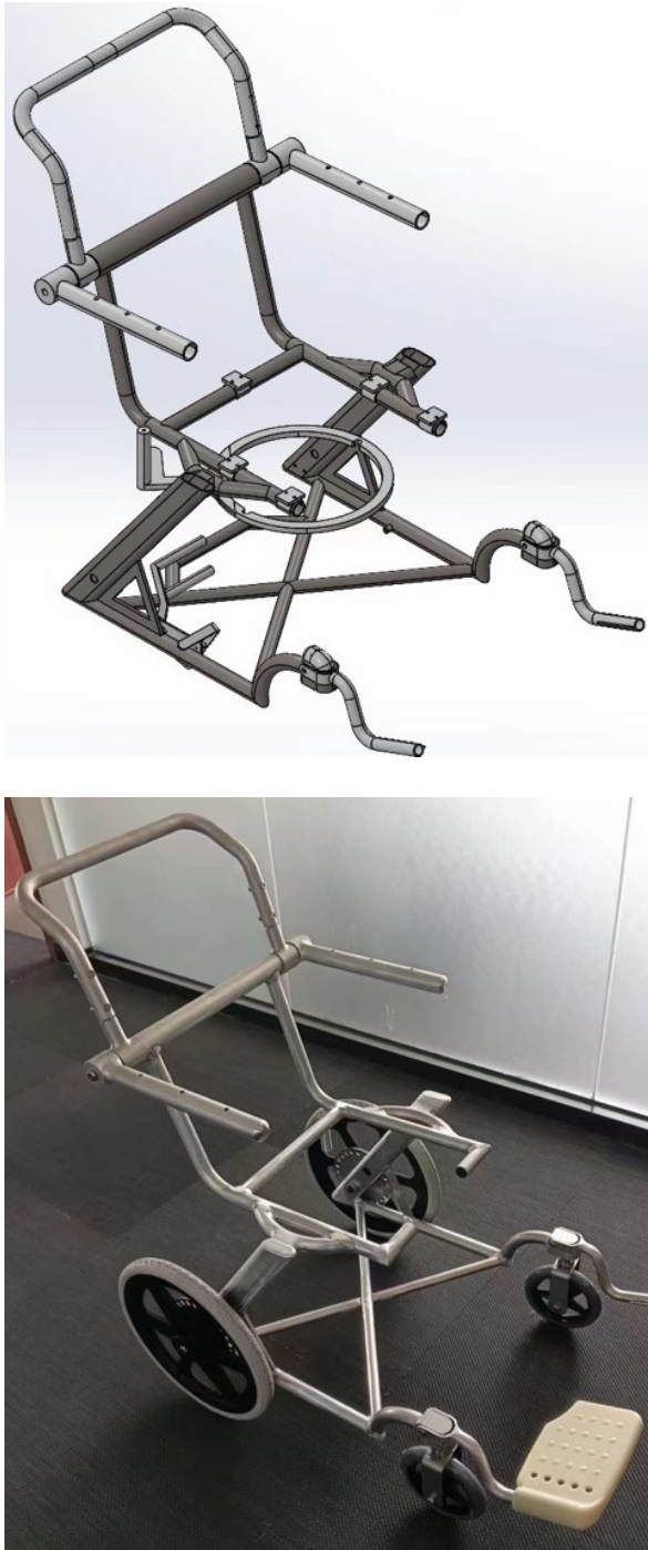
Figure 27. Structure Design: 3D CAD Model (Left) and Prototype (Right)
