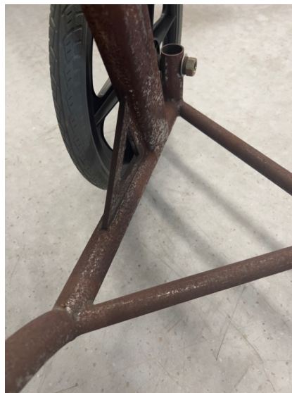
Figure 25. Rust on the Steel Structure Frame
