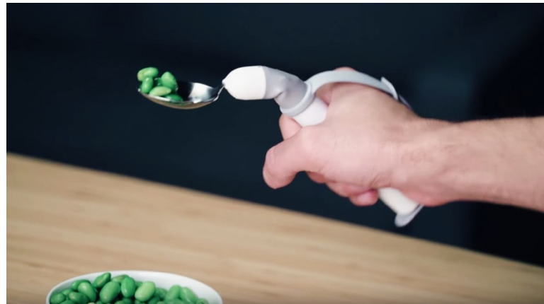
Figure 2. A Self-Stabilising Smart Spoon
