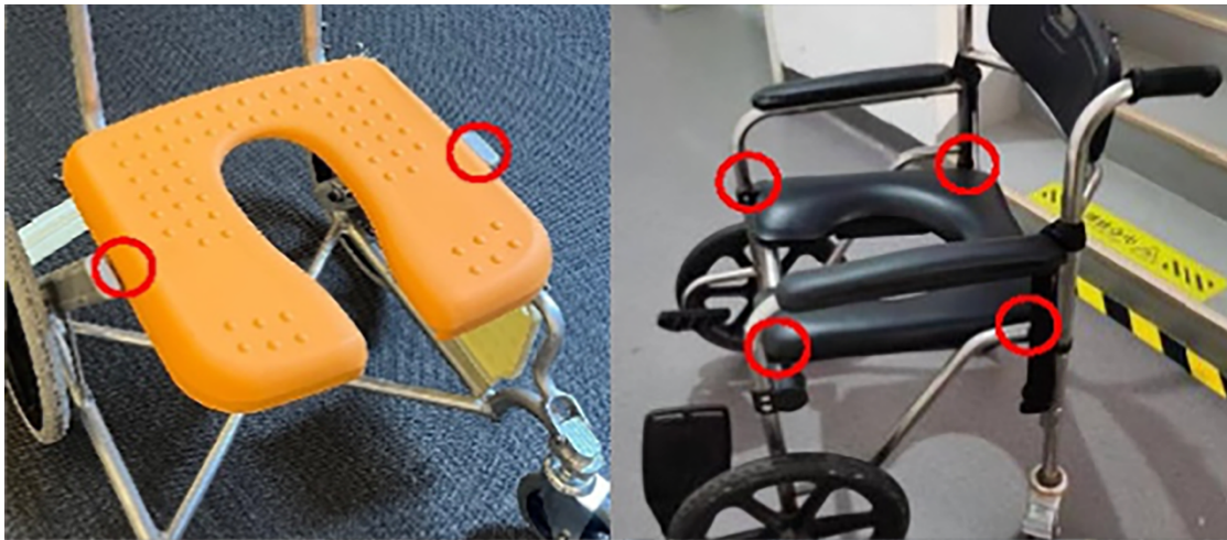
Figure 30. Comparison of Mounting Points: Prototype (Left) and Conventional (Right) Shower Chair
