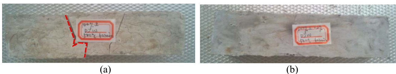
Figure 2 Cracking in geopolymer specimens a without CF and b with 2% CF after exposure to 500°C [11].
