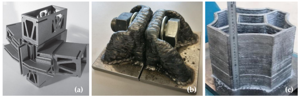
Fig. 13 AM connection examples: a Nematox facade (Strauss et al. 2015), b T-stub (Erven et al. 2021) and c space frame (Lange et al. 2021)
