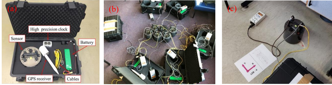
Figure 4 (a) A set of equipment used in the field test; (b) ‘huddle test’ by placing sensors together to check the status of the instruments; (c) on-site view of the equipment.
