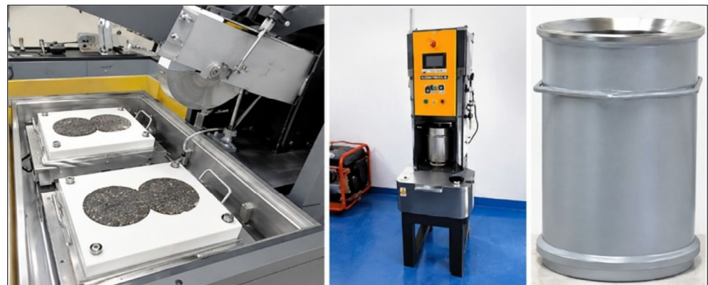
Figure 11. WMA Specimens' Production in Accordance with AASHTO T312.
