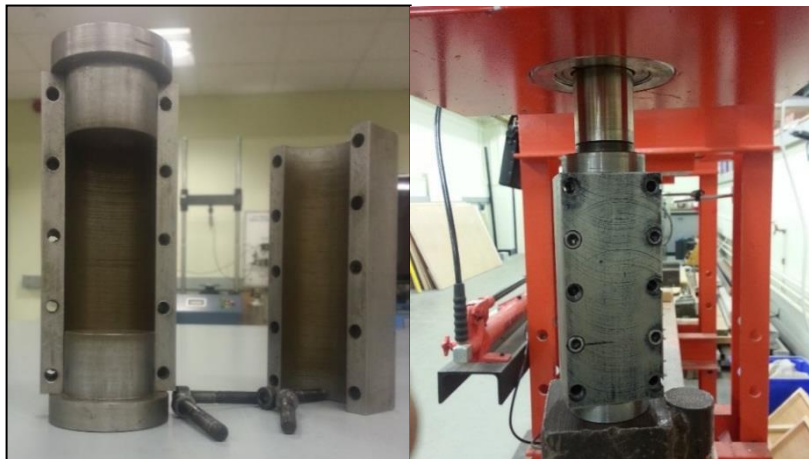
Figure 5. Constant volume mould and the hydraulic jack
