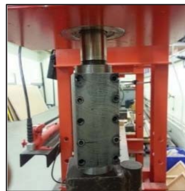
Fig. 4 Preparing of UCS test specimens
