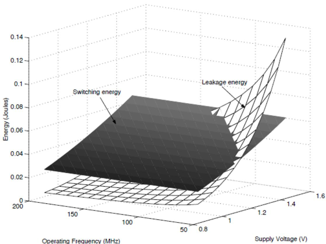
Figure 3.7 Comparison of leakage and switching energy in SA-1100 (Sinha and Chandrakasan 2000).
