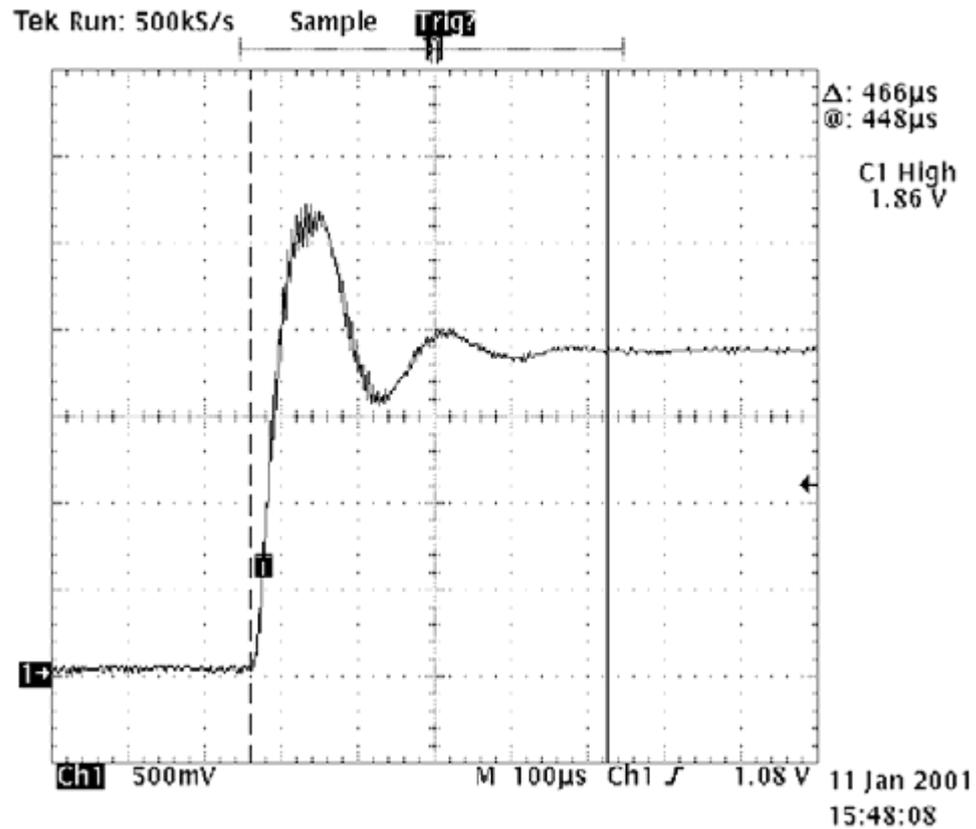
Figure 3.5 466 µs startup transient from the µAMPS-1 2.4 GHz radio, measured at the input to the radio's VCO (Min 2003).
