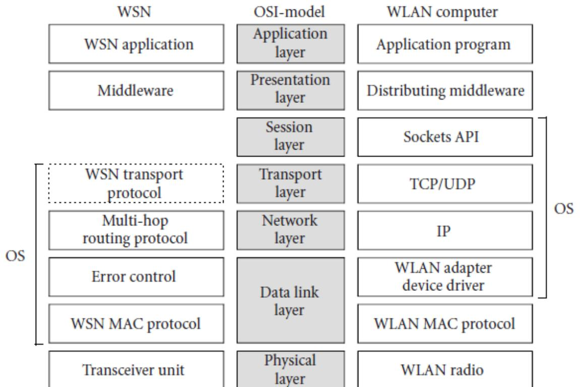
Figure 3. 10 OSI model, WSN, and distributed system in WLAN protocol layers (Kuurilehto et al. 2005).
