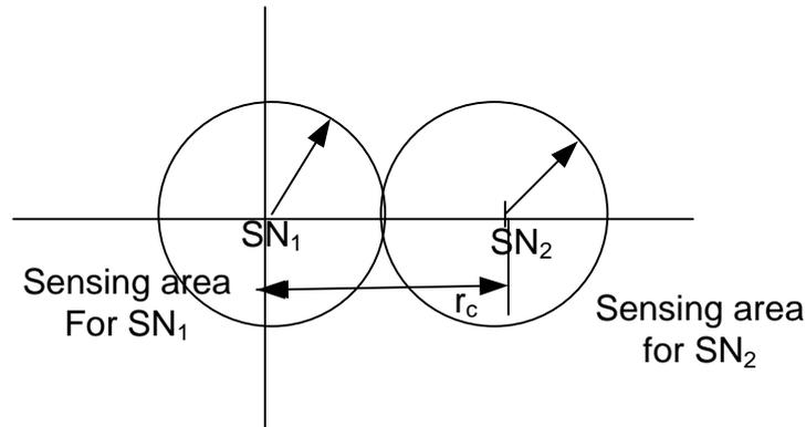
Figure 3.3 Sensing and Communication range of SNs
