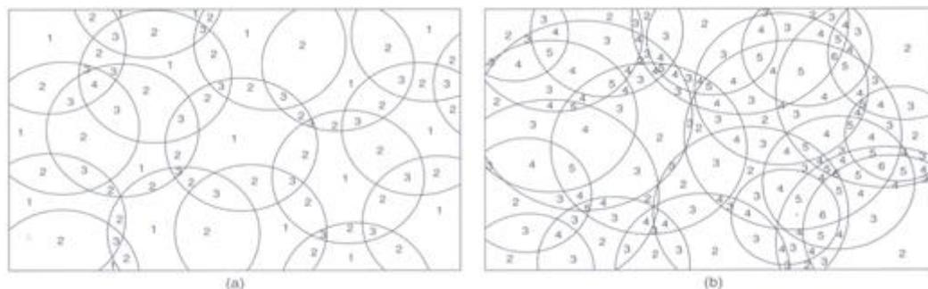
**Figure 2. 1 Example of the coverage problem: (a) a sensing field which is 1-covered by unit disks and (b) a sensing field which is 2-covered by non-unit disks. The number in each sub-region is its coverage level (Wang et al. 2003).**
