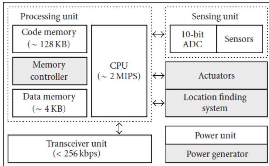
Figure 3. 8 Reference hardware platform architecture of a sensor node (Kuorilehto et al. 2005).
