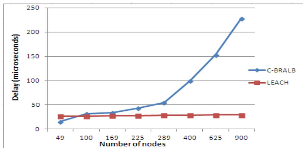
Figure 6. 17 Average packet delay of C-BRALB vs. LEACH
