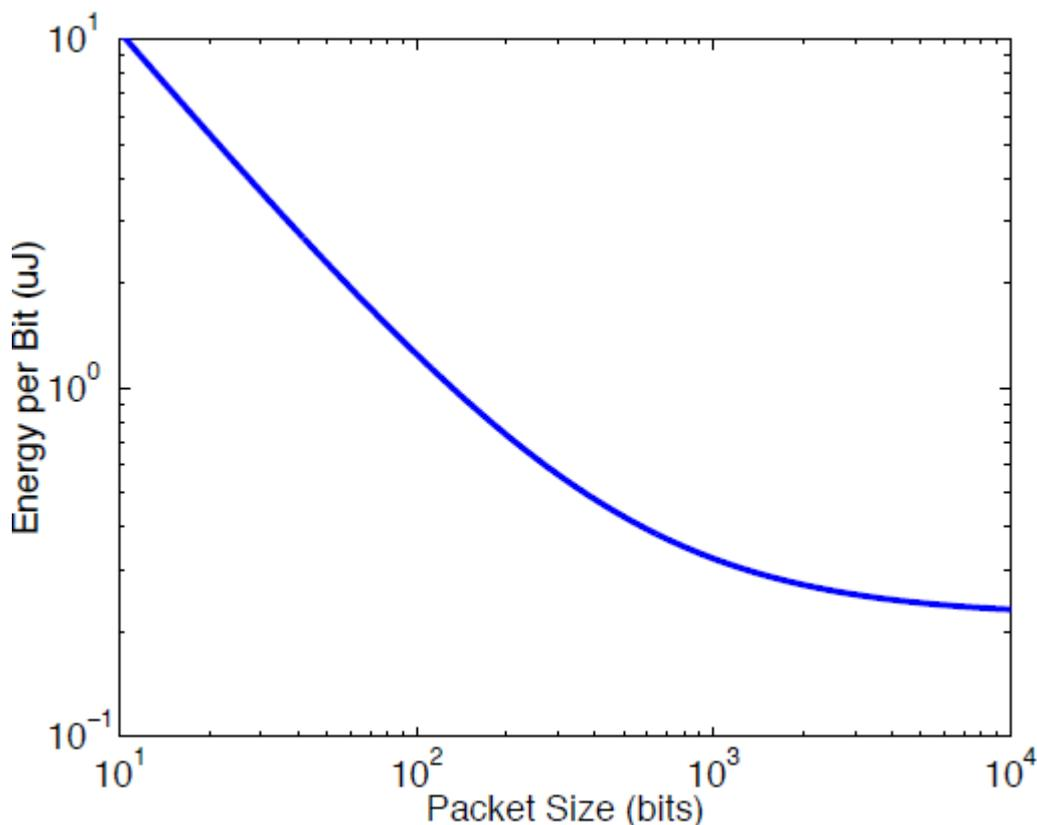
Figure 3. 6 The total radio energy per bit required to transmit packets of various sizes. The radio has a data rate of 1 Mbps, start-up time 466  $\mu s$ , and the active transmitter electronics consume 220 mW (Min 2003).
