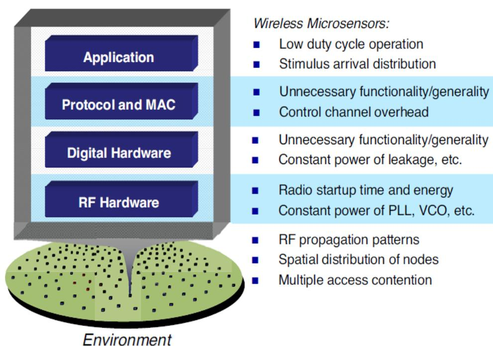
Figure 3.4 Sources of inefficiency in communication across the system hierarchy (Min 2003).
