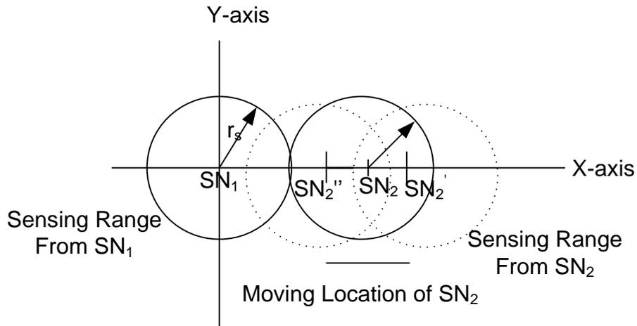
Figure 3. 2 Sensing Range of a SN
