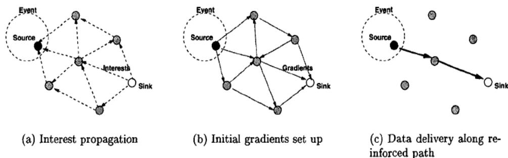
Figure 4. 1 A simplified schematic for directed diffusion (Intanagonwiwat et al. 2000).
