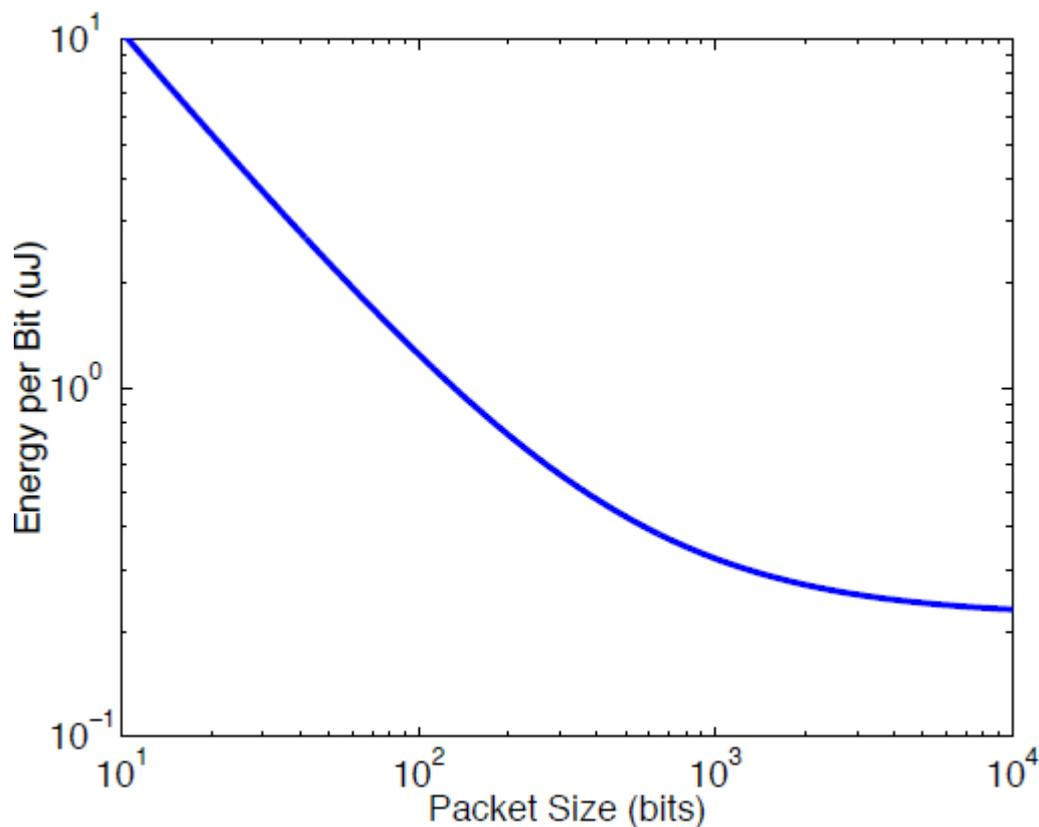
Figure 3. 6 The total radio energy per bit required to transmit packets of various sizes. The radio has a data rate of 1 Mbps, start-up time 466  $\mu\text{s}$ , and the active transmitter electronics consume 220 mW (Min 2003).
