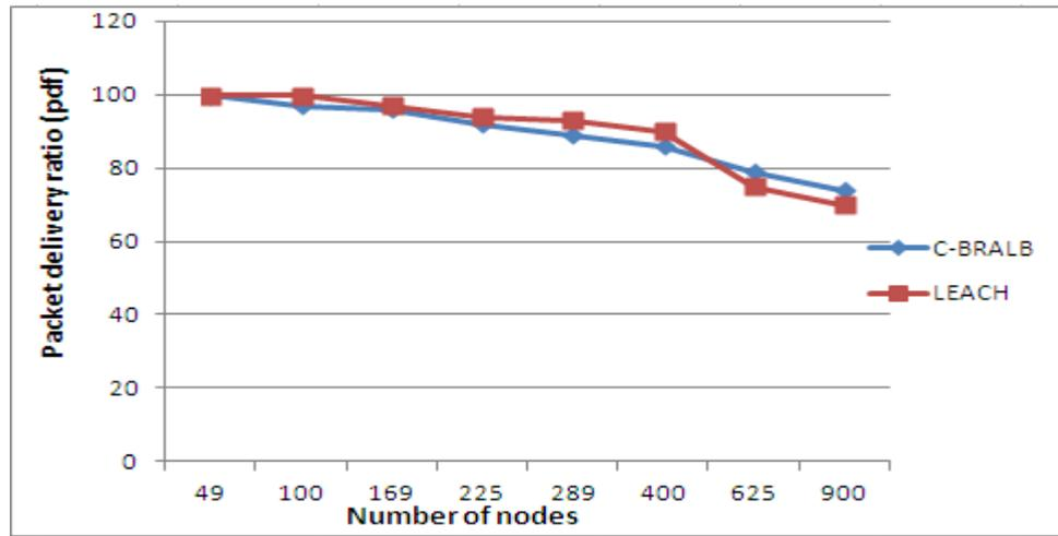
Figure 6. 16 Packet delivery ratio of C-BRALB vs. LEACH
