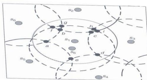
**Figure 2. 2 A WSN example where sensor  $s_1$  locally decides itself to be redundant and hence goes to sleep based on the approach proposed (Wang et al. 2003).**
