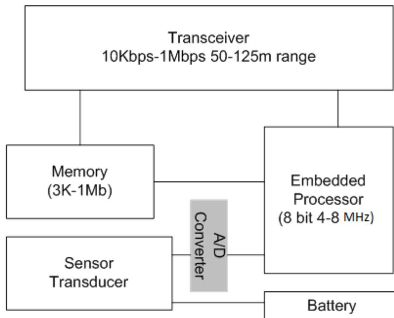
Figure 3. 1 Functional Block Diagram of a typical Sensor Node (Biswas et al. 2005)
