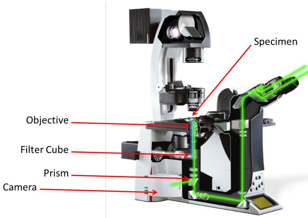
**Figure 3.11.** Schematic representation depicting the path of excitation and emission light in a fluorescence microscope. Excitation light (blue) is directed onto the sample via the objective. The fluorophore is then excited and emits fluorescence (green). The green light is passed through a prism filtering out light of other wavelengths and produces an image that can be seen through the eyepiece or camera of the microscope.
