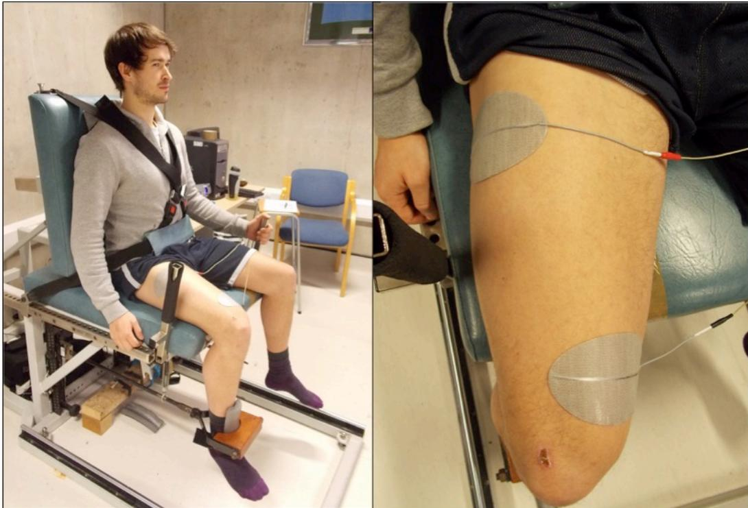
**Figure 4.2.** EMS experimental set up. Left: participant fully secured in the isometric chair. Right: placement of the electrodes used to deliver electrical stimuli.
