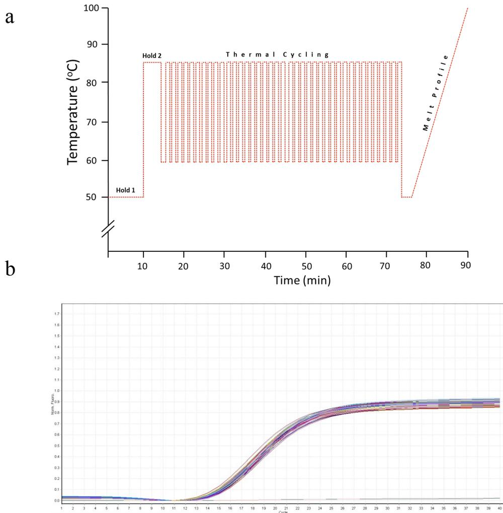
**Figure 3.5.** a) Design of the polymerase chain reaction protocol used in the experiments described in this thesis. b) examples of real time fluorescence detection curves. Cycle threshold is determined from this curve by locating the lower third of the curve below the exponential phase of amplification.
