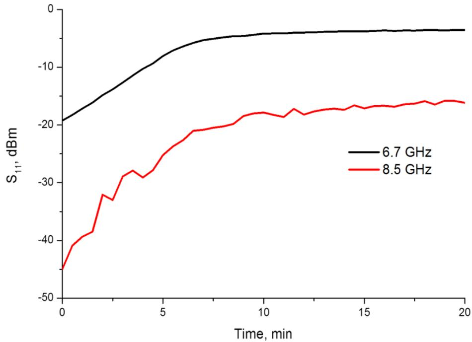
Figure 59: Dependences of  $S_{11}$  signal amplitude versus time at two selected frequencies, namely 6.7 GHz and 8.5 GHz, which can be used as a calibration curve for the real-time monitoring of glue settling state and industrial process optimization.
