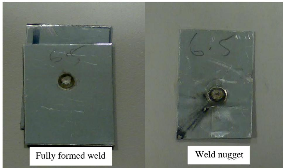
Figure 8: Good quality spot weld nugget at 6.5kA before and after the peel test
