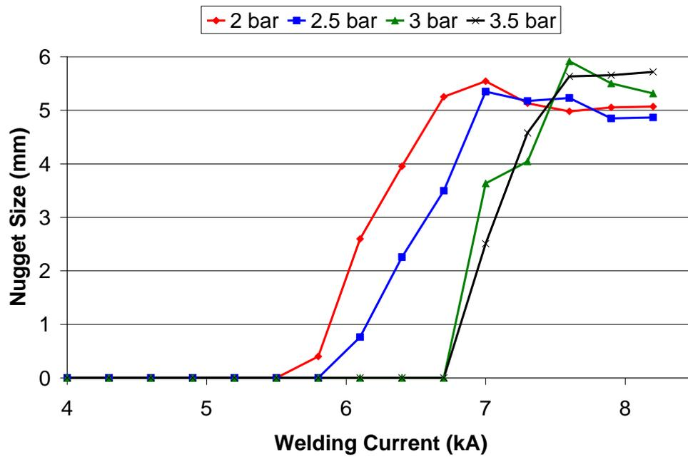
Figure 37: Weld growth curves for different electrode forces for coated mild steel
