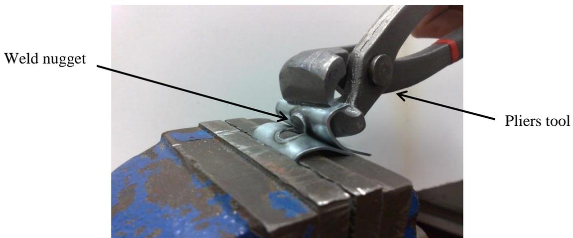
Figure 5: Destructive Spot Welding Offline
