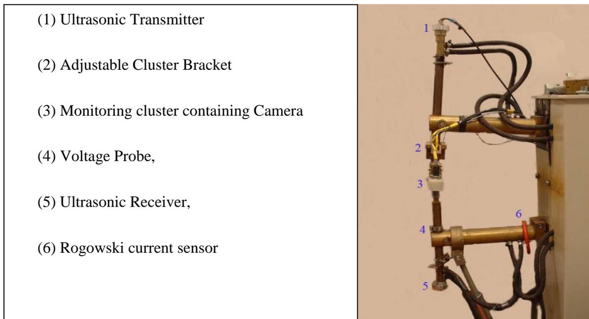
Figure 7: The Experimental sensors setup
