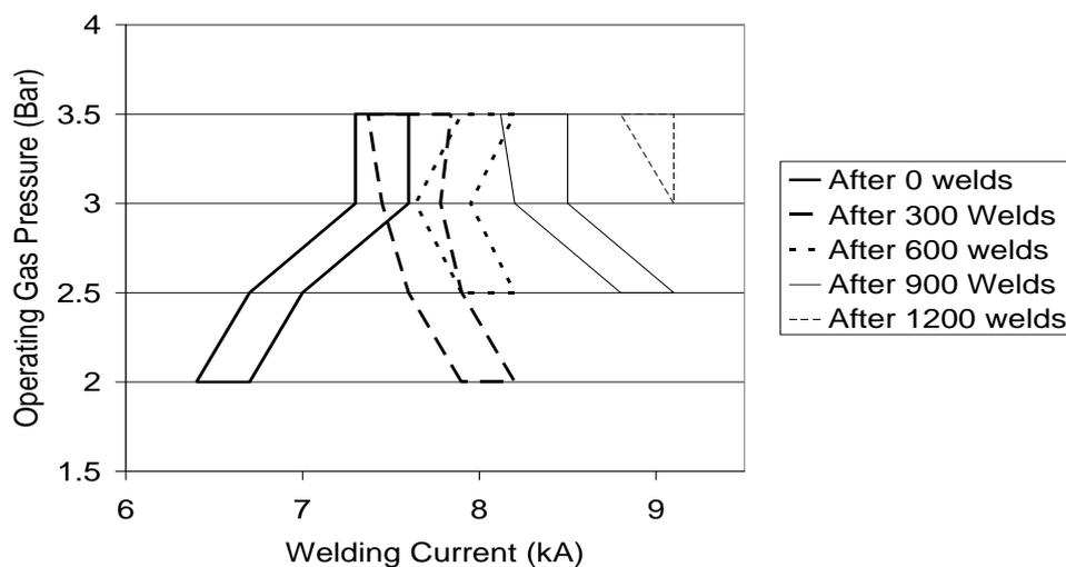
Figure 39: Weldability lobes for an increasing number of welds
