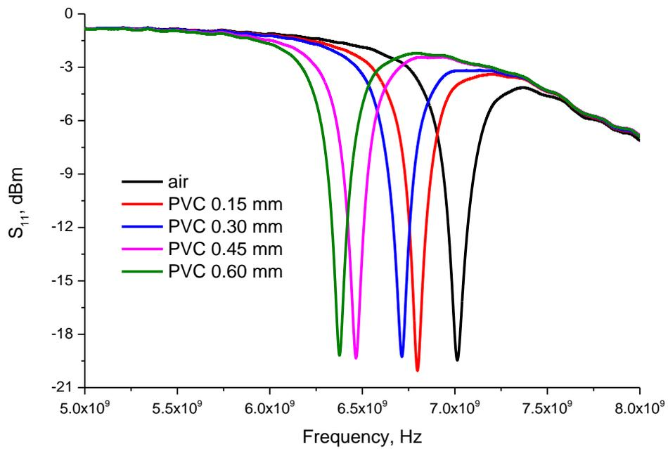
Figure 53: Dependence of  $S_{11}$  signal on the thickness of PVC, placed on top of the sensor with Au pattern on FR4 substrate, 5.0-8.0 GHz range.
