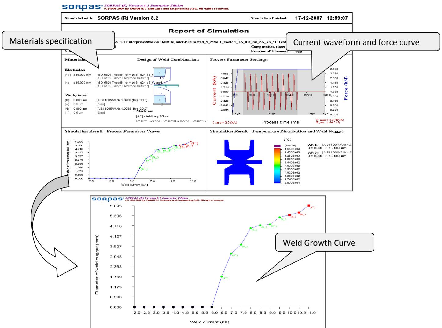
Figure 26: Representation of the welding profile, including materials specifications, current profile, weld growth curve profile
