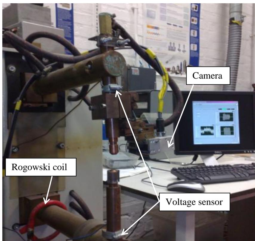
Figure 28: The Experimental sensors setup
