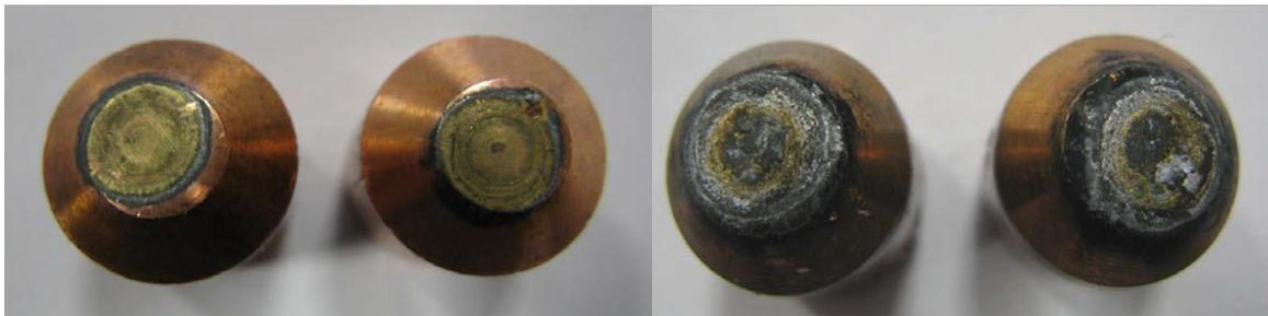
Figure 9: Deterioration of Electrode Tips
