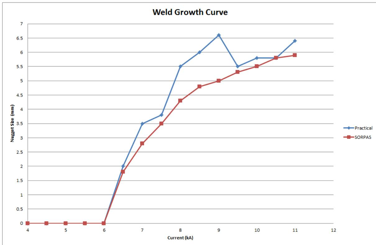
Figure 47: Theoretical and Practical representation of the weld current vs. the diameter of the weld nugget
