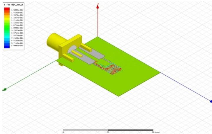
Figure 50: HFSS model of microwave sensor field.
