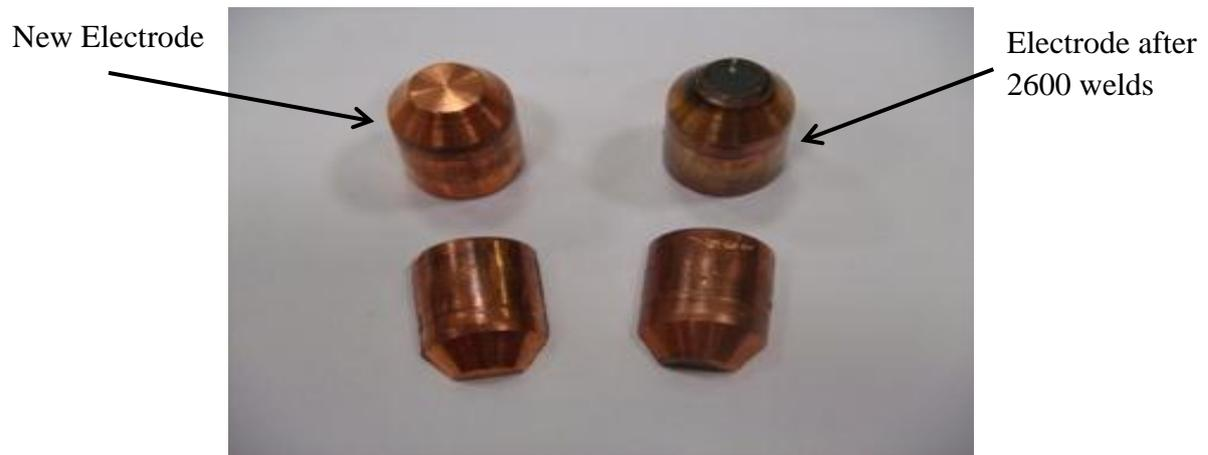
Figure 18: New Electrode Tips and Degraded Electrode Tips (after 2600 welds)
