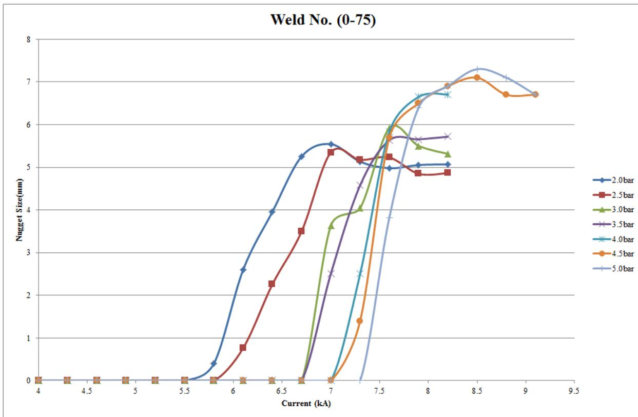
Figure 41: Points out practical representation of different pressures on a brand new tip
