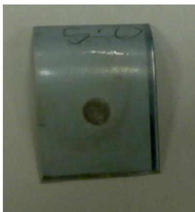
Figure 29: No weld after destructive testing
