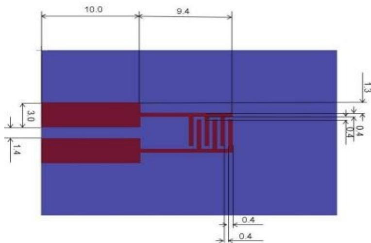
Figure 48: A printed Au pattern layout: all dimensions are in mm
