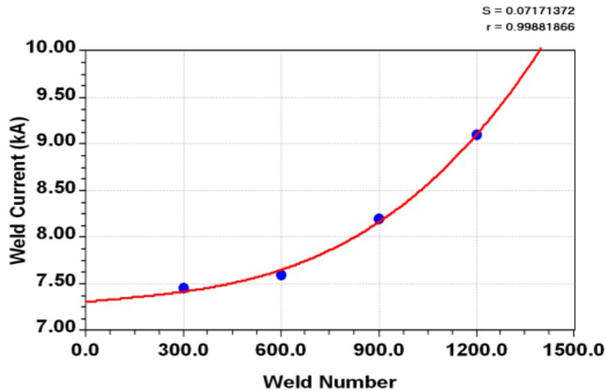
Figure 40: Curve fitting algorithm output for minimum current
