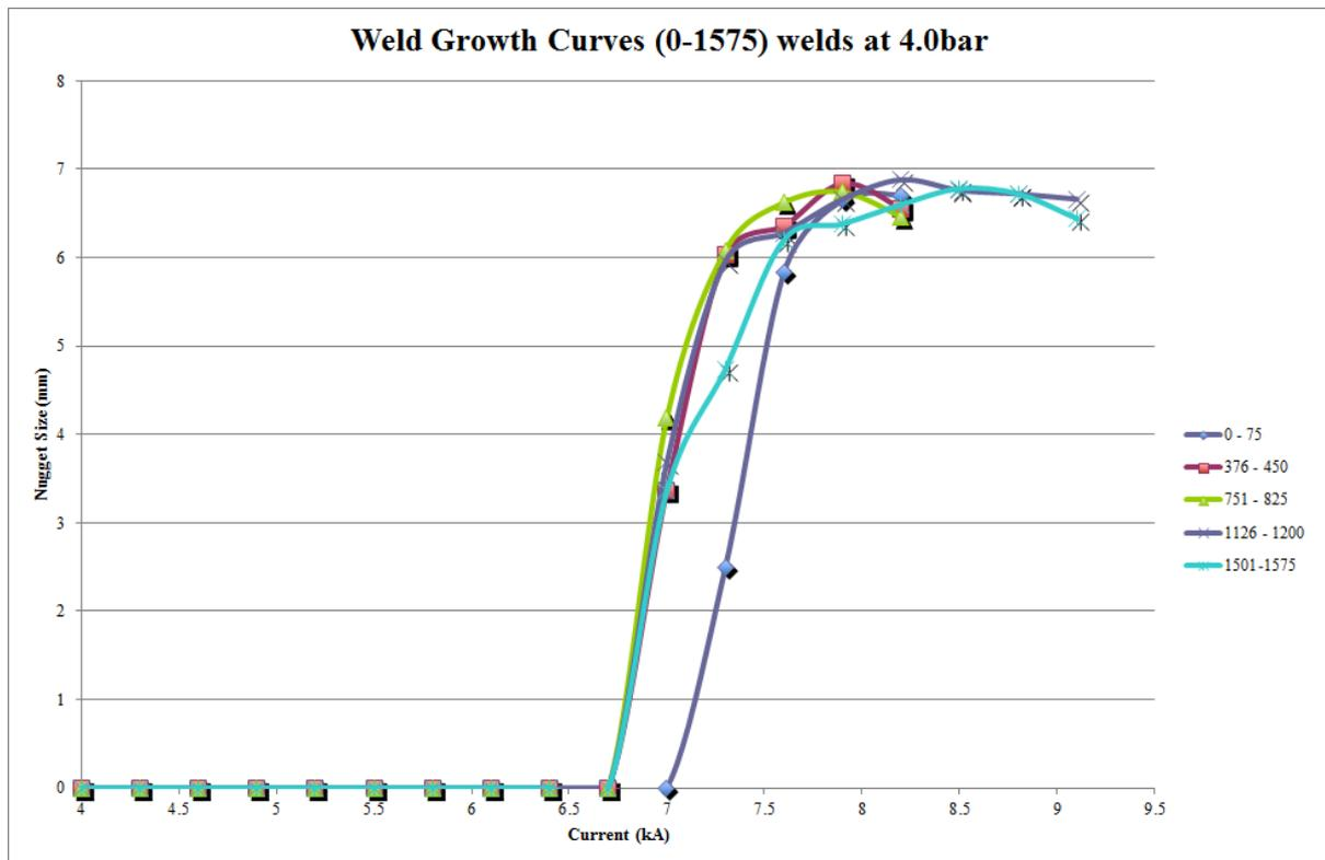
Figure 46: Practical representation of the weld current vs. the weld nugget diameter at 4.0bar
