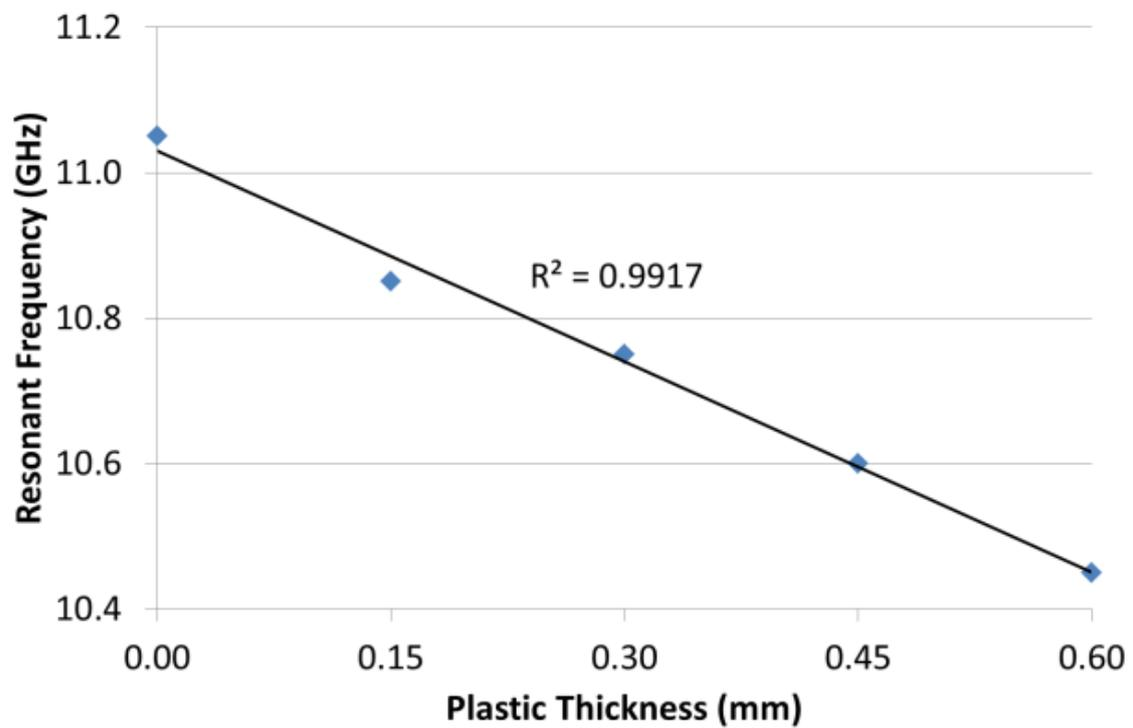
Figure 54: Change in the resonant peak frequency with the thickness of PVC in contact with the EM wave sensor.
