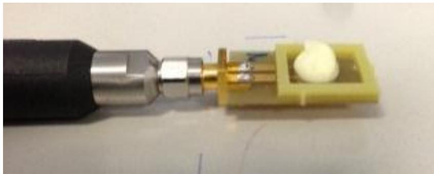
Figure 57: PF glue sample placed on the microwave sensor
