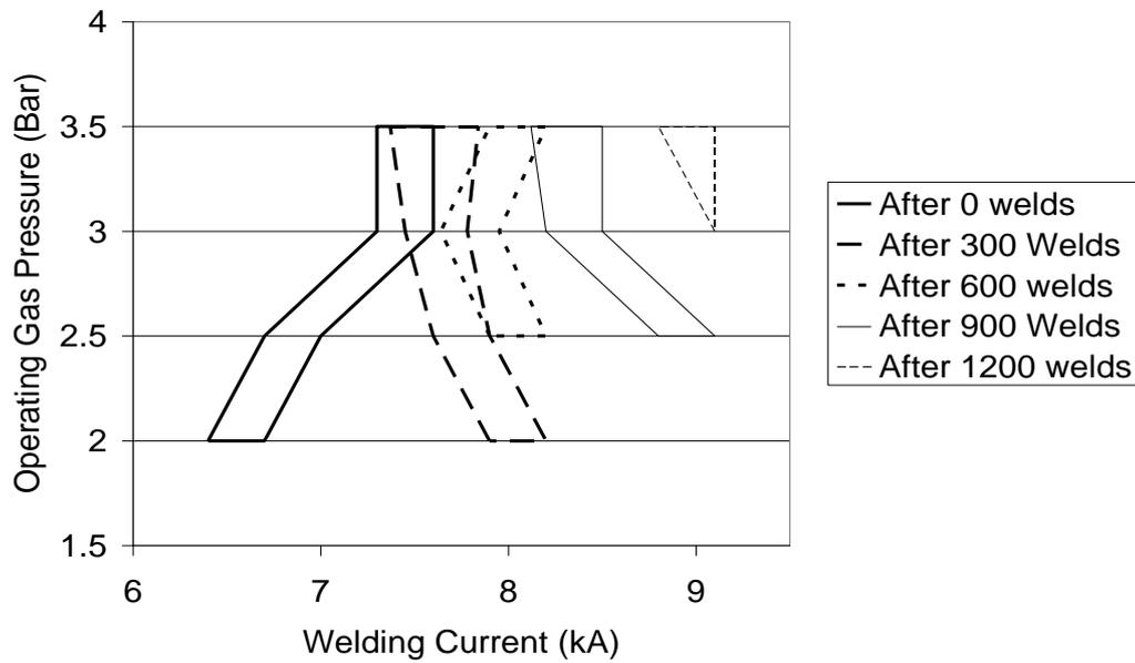
Figure 19: Representation of weldability Lobe for coated 0.8mm steel [54]
