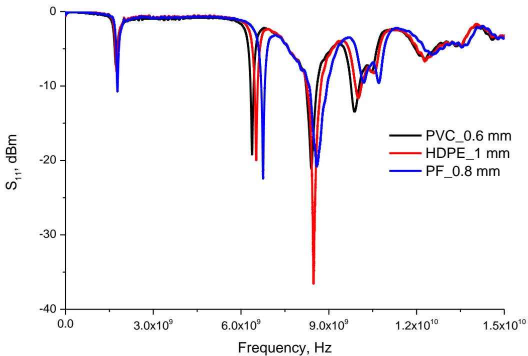
Figure 56:  $S_{11}$  signal dependence on the material type brought in contact with Au pattern on FR4 substrate, 0.1-15 GHz frequency range.
