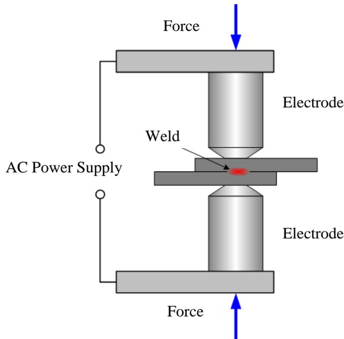
Figure 1: The pressure and the current are usually applied via the same electrodes
