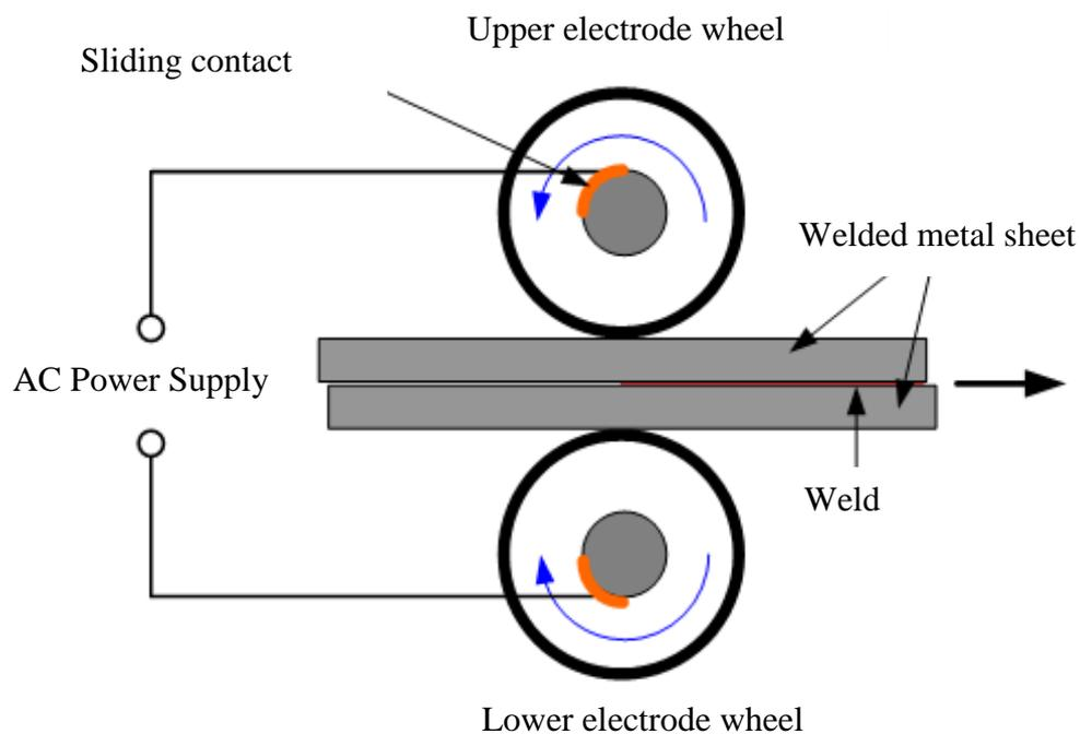
Figure 11: Resistance Seam Welding [34]
