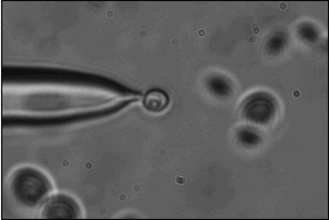
*Figure 7-26 optically trapped yeast cell elevated above the general population of cells demonstrating 3D trapping in the process*
