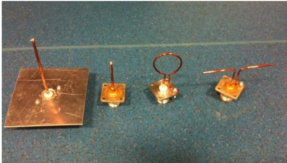
Figure 43 Antennas built for experiments (from right to left: one wavelength monopole with ground, a half wavelength monopole, one wavelength loop and one wavelength dipole)
