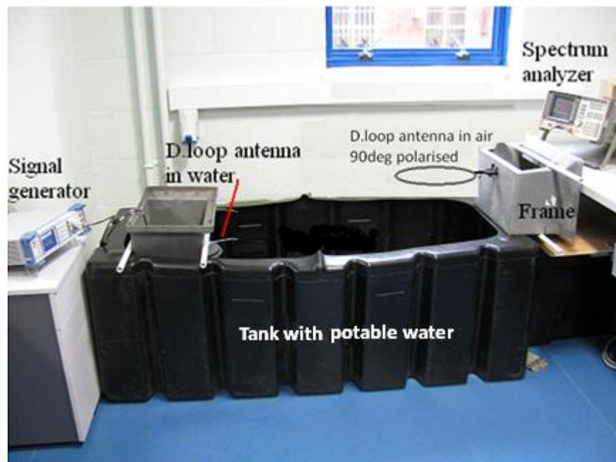
Figure 39 Experimental setup at ISM frequencies with double loop antennas
