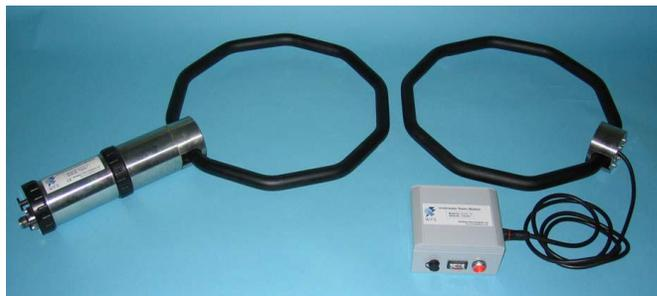
Figure 9 Underwater radio S1510 transmitter and receiver [64]
