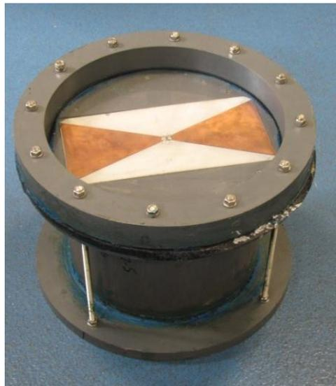
Figure 107 Underwater transmitter
