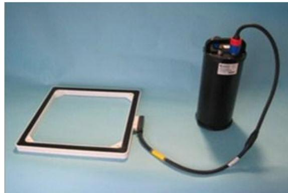
Figure 11 Underwater radio modem Seatooth S300 [64]
