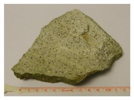
Figure 25: Photograph of sample 29 (site 14), porphyritic rhyolite with fiamme structures (pale parallel lines).
