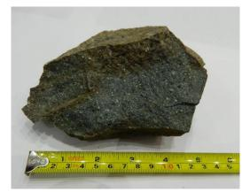
Figure 23: Photograph of sample 2 (site 1), porphyritic rhyolite.
