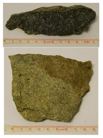
Figure 32: A: Photograph of sample 30 (Site 16), gabbro from the central sheeted unit. B: Photograph of sample 31 (site 16), granite from the central sheeted unit.
