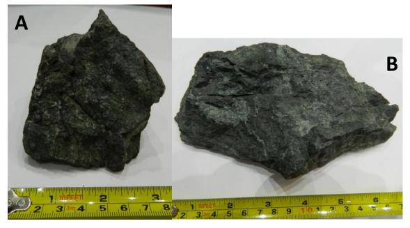
Figure 20: A: Photograph of sample 1 (site 1), basalt. B: Photograph of sample 3 (site 1), basalt showing fine calcium carbonate veins.
