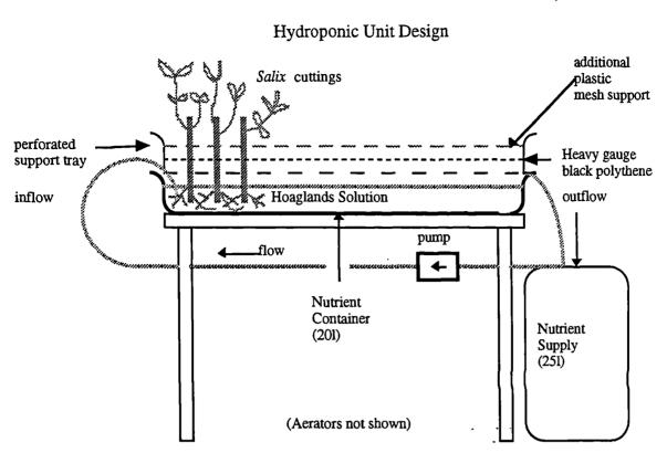
Figure 1. The suspension hydroponic system used in the following study.
