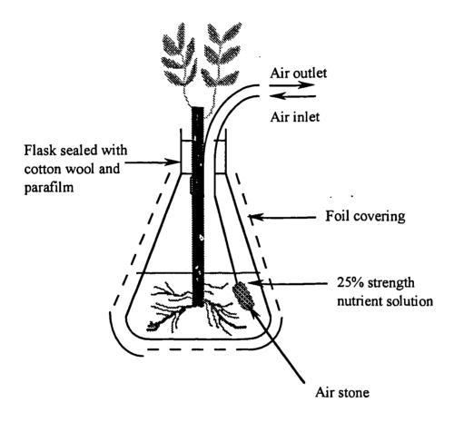
Fig. 1.0. Set up of single flask solution culture units.
