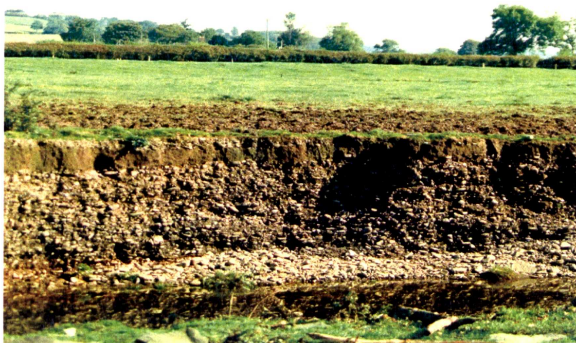
Figure 3.8 Oblique view (June 1998) of a composite, erosive bank face in the Chapel View study reach. The bank face is approximately 1.5 m high.
