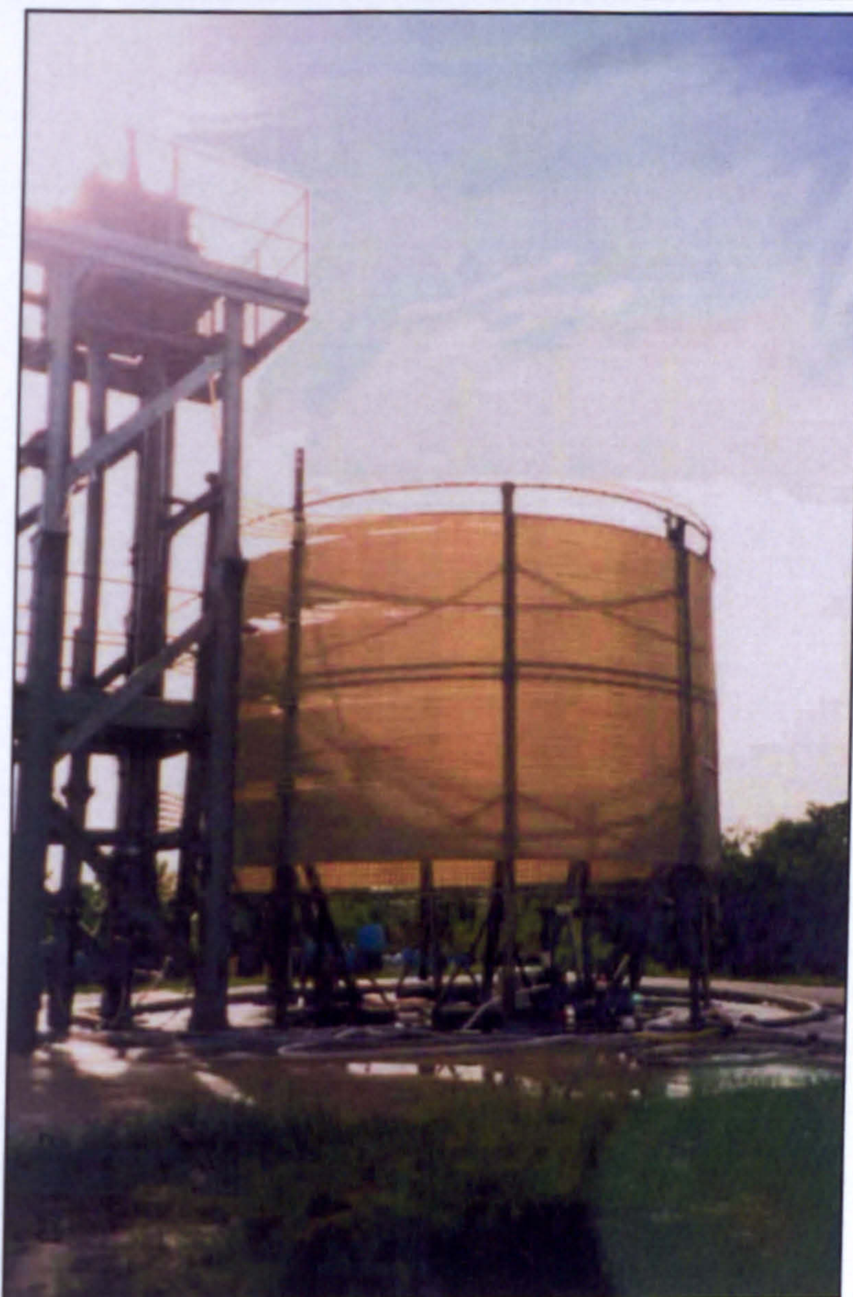
Plates 12: A 2000 L helical photobioreactor. A 70L culture to the bottom right showing comparative scale (top). Inner diameter of the 2000 L photostage is 5.25 m. A covering was used during inoculation with I. galbana (data not shown) to prevent photoinhibition during early growth. This was removed once cell density had risen (bottom). Location: Harbour Branch Oceanographic Institute (Fort Pierce, Florida, USA).
