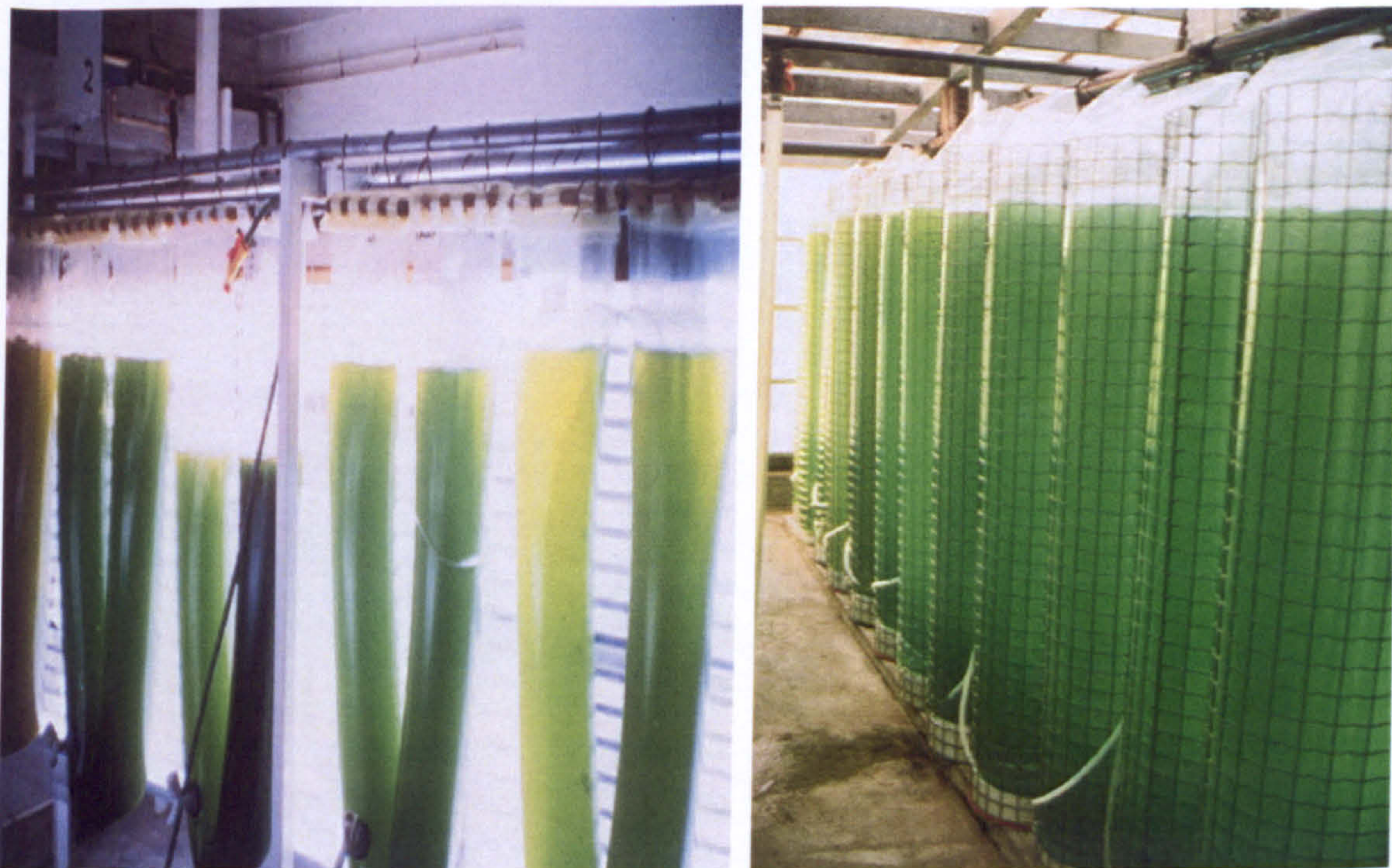
Plate 3: 'Poly-bag' cultures. Polyethylene bags filled with culture hung from a beam (left). Cultures can be grown indoors although artificial lighting is required (left). A tube is inserted from top to bottom in order to mix and aerate cultures. Larger bags (right) can hold up to 500 L, and are supported using a plastic base and wire mesh.
