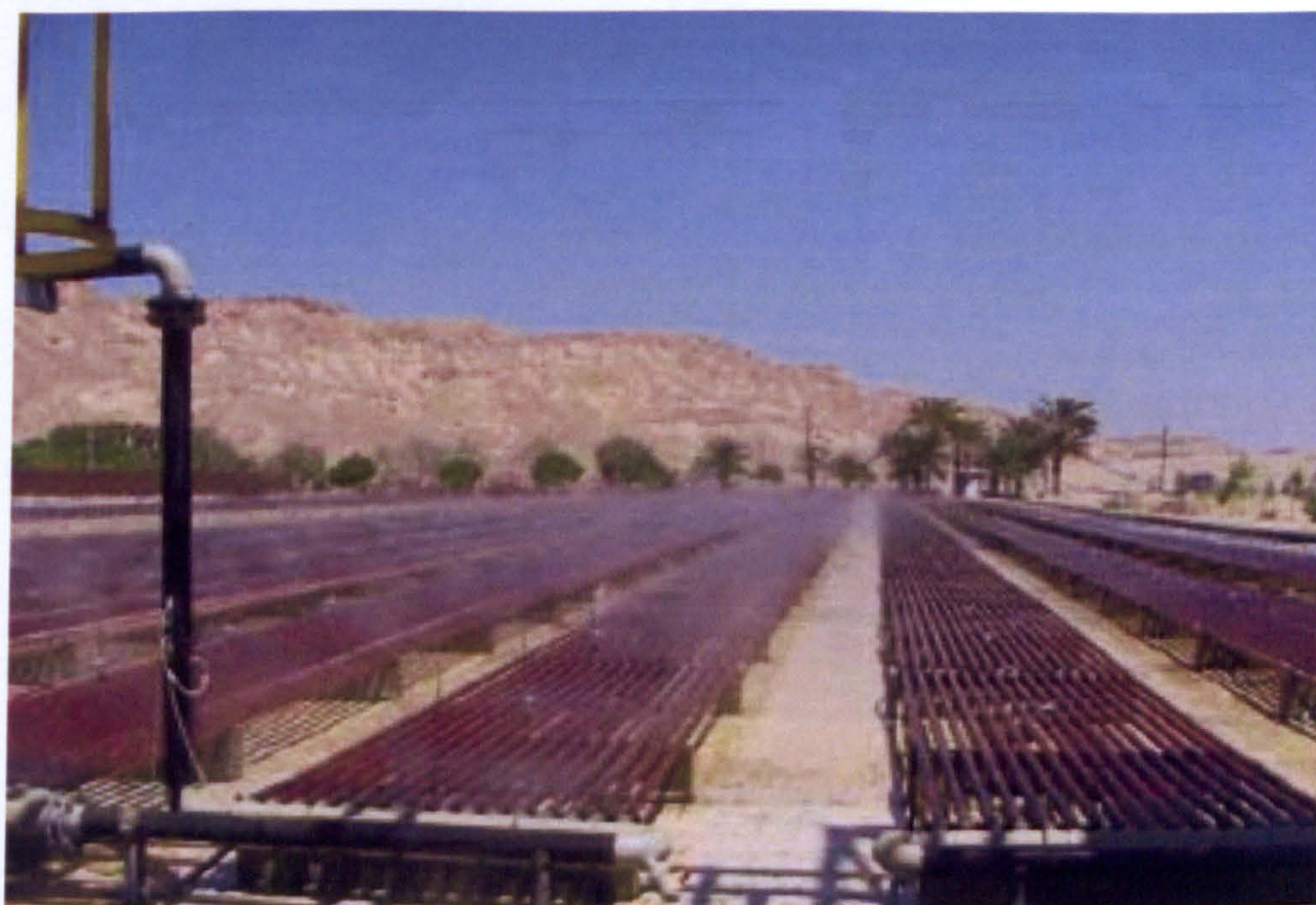
Plate 5: A horizontal tubular photobioreactor with manifolds. This system based in Sede Boqer, Israel. Developed by the Jacob Blaustein Institute for Desert Research, the downcomer is devised into parallel rows, which are more energetically efficient for recirculation.
