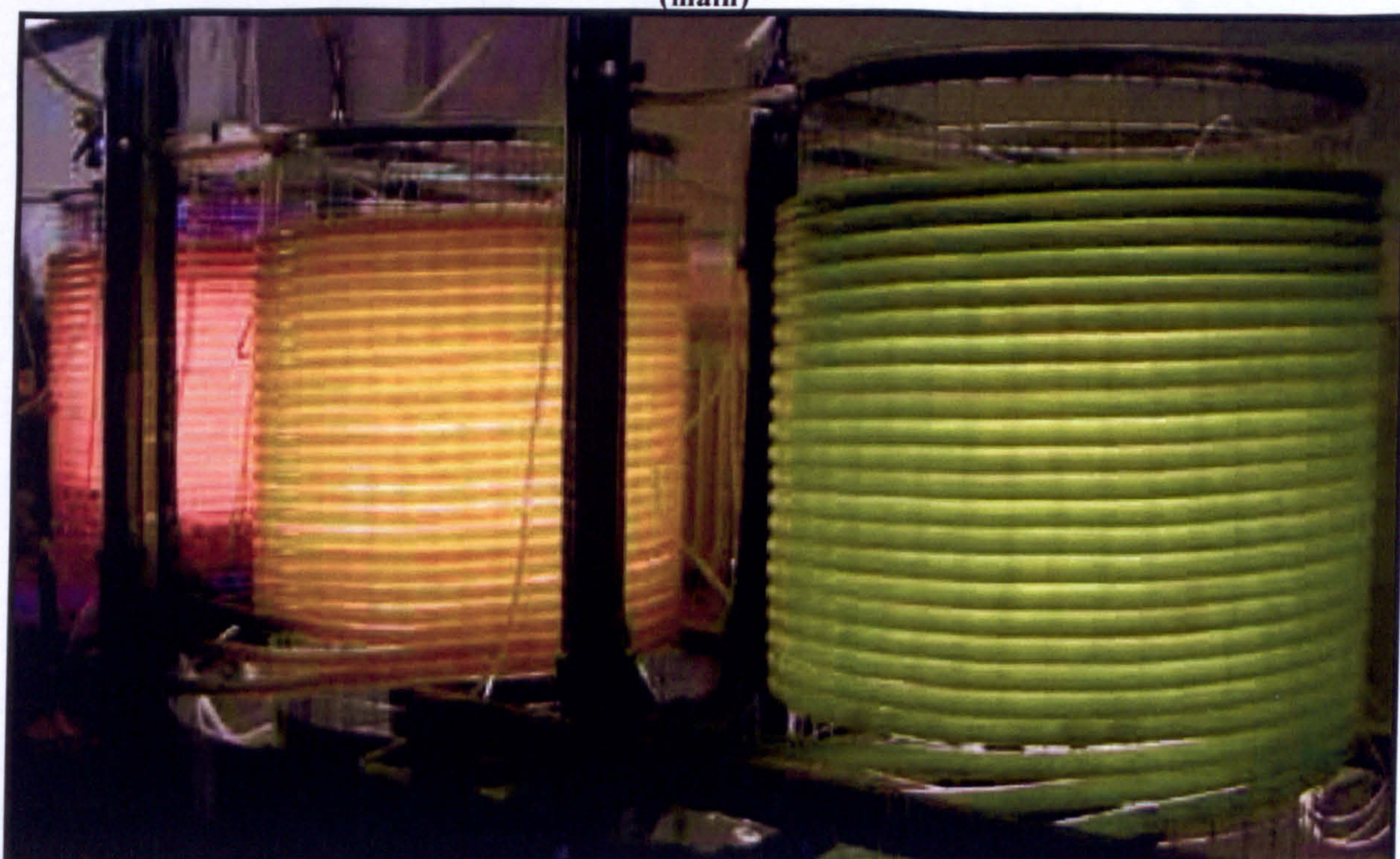
Plate 6: 70 L indoor tubular photobioreactors. Plates 6a and 6b show various sections of the photobioreactor used in this study for cultivation of I. galbana (left) and N. oculata (right). See also Figures 3.1 – 3.5 and Appendix C for measurements. The bottom picture shows a close up of photostages of three different caultures: Tetraselmis sp. (left- data not shown), I. galbana (centre) and N. oculata (right).
