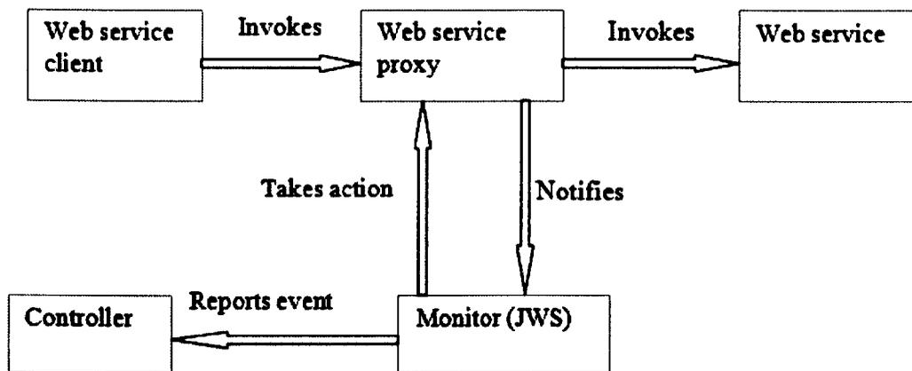
**Figure 5.8: An interaction model for autonomic Java web services (proxy with embedded sensor and actuator).**
