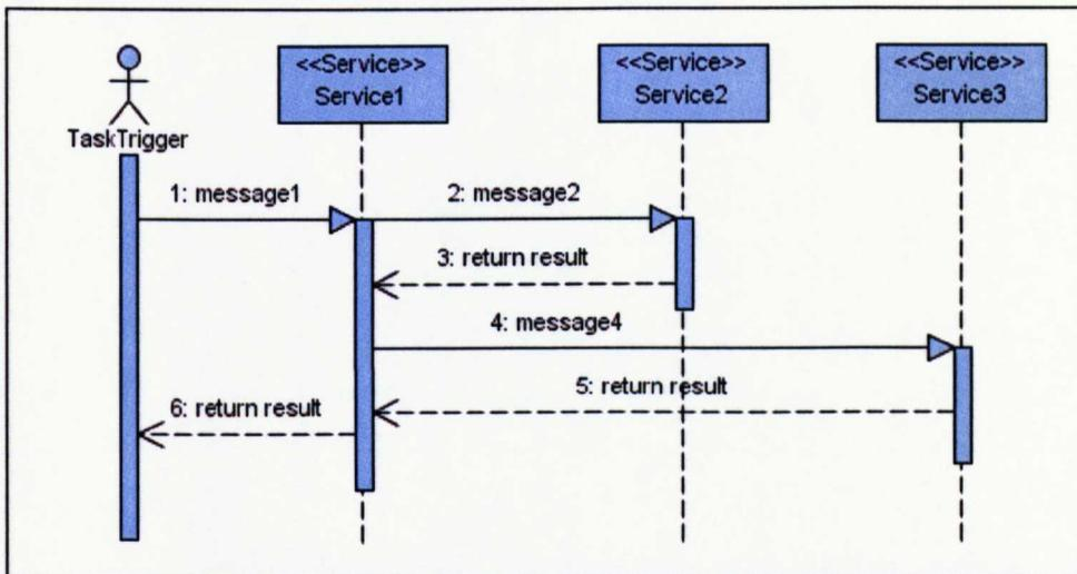
**Figure 5. 3:** The required services for a particular task.
