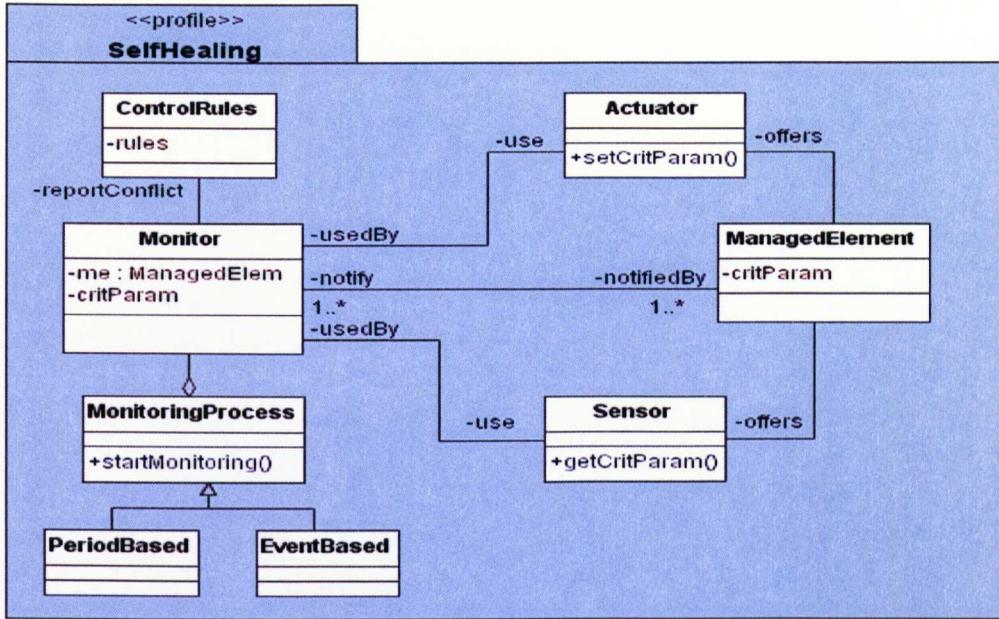
Figure 5. 6: Simplified UML profile for self healing systems.
