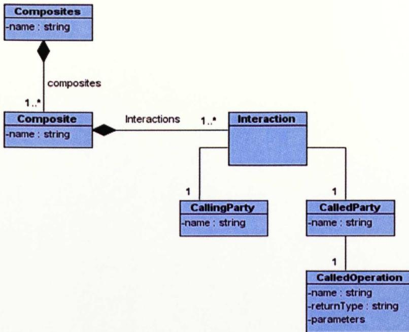
Figure 5.5: The class diagram for XML schema of the composite file.
