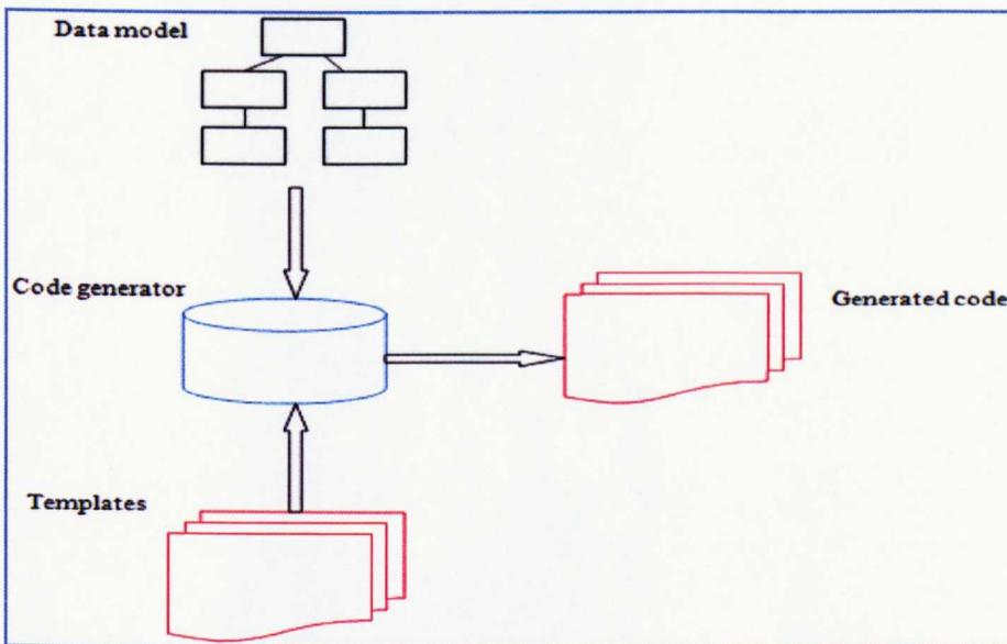
**Figure 6.4: The Template based code generation process.**
