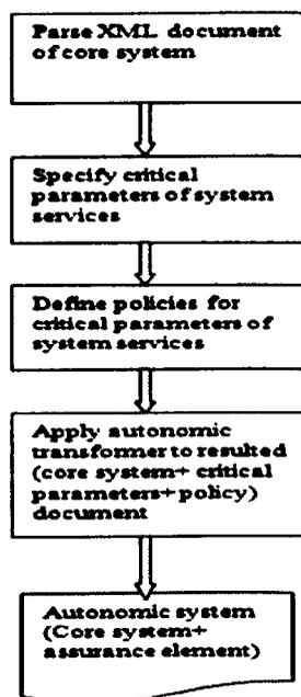
**Figure 6.1: Application of autonomic transformer to core system.**
