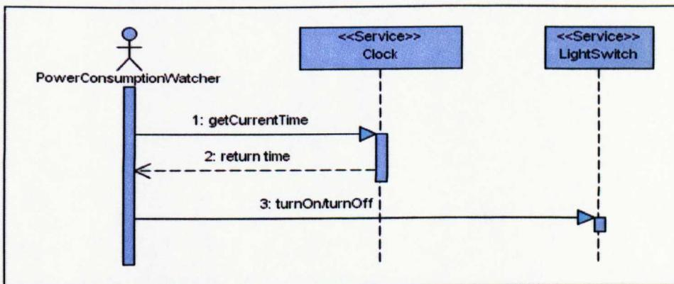
Figure 8.18: Services for 'Ensure efficient power consumption' task.
