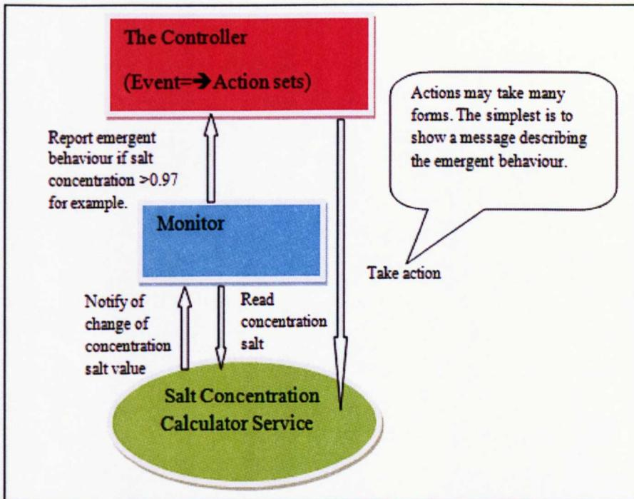
**Figure 8. 38: The Service-Monitor-Controller design style for the salt world domain.**
