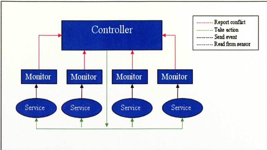
**Figure 5.10: The Service-Monitor-Controller (SMC) style for autonomic systems.**
